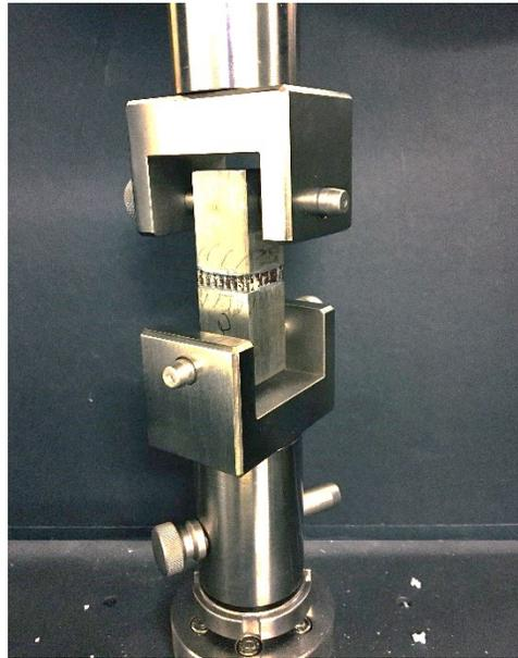
*Figure 3.11: Sample subjected to flatwise tensile loading.*
