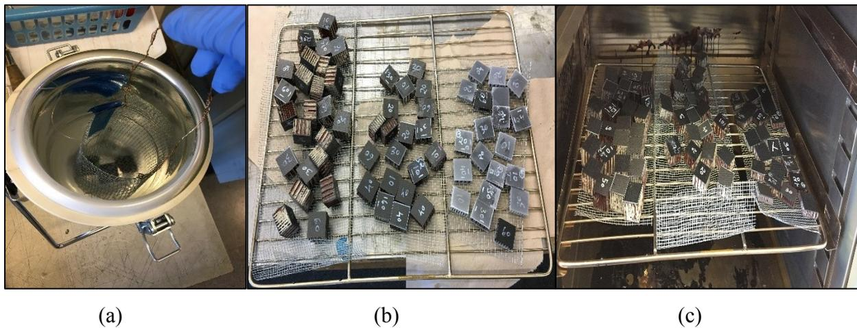
*Figure 4.2: (a) Samples dipped in LN<sub>2</sub>, (b) Samples at room temperature, (c) Samples placed in convection oven*
