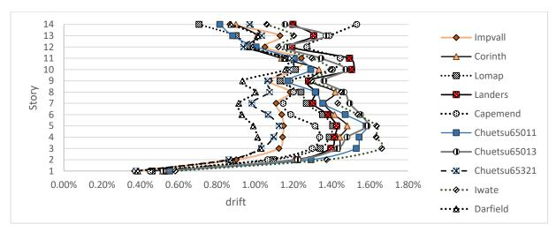
Figure 4-17 Time History drift for moderately- ductile model with dampers (MD-D)
