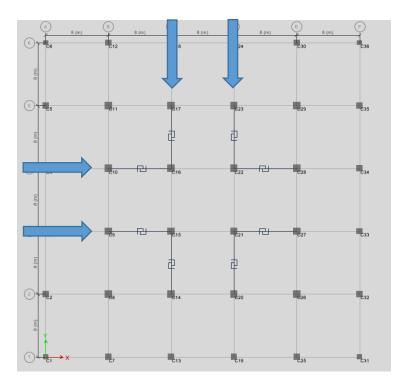
Figure 2-5 Floor view and dampers directions
