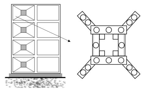
Figure 1-3 friction dampers installed in X braces in a structure
