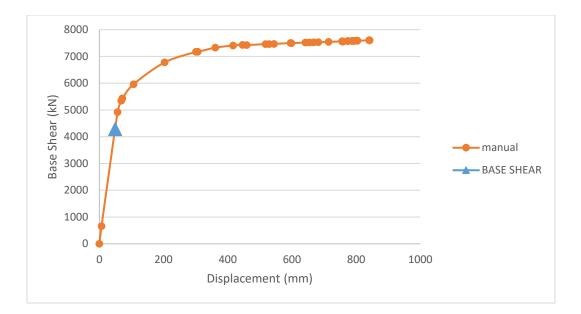
Figure 4-7 Pushover curve for Ductile building (DUC)
