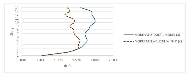
Figure 4-19 Standard deviation + Mean value Drift for time History analysis model (MD) & (MD-D)
