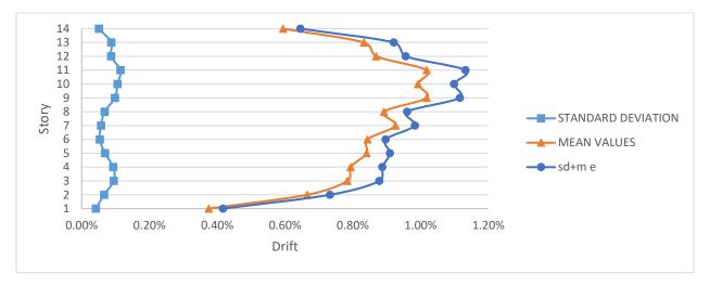
*Figure 4-13 Standard deviation, mean values and sum for the Time History drift for elastic model with dampers (EL-D)*
