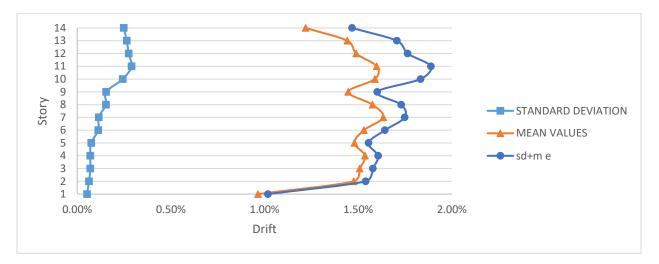
Figure 4-23 Standard deviation, mean values and sum for the Time History drift for ductile model with dampers (DUC-D)
