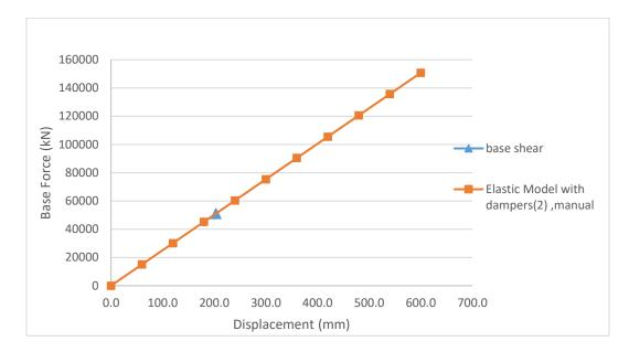
Figure 4-1 Pushover curve for Elastic building (EL)
