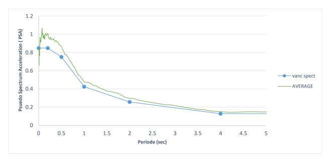
Figure 2-13 Average Ground-motion matching Vancouver Spectrum
