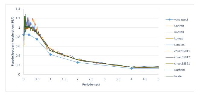
Figure 2-12 10 Ground-motion matching with Vancouver spectrum (5% damping)
