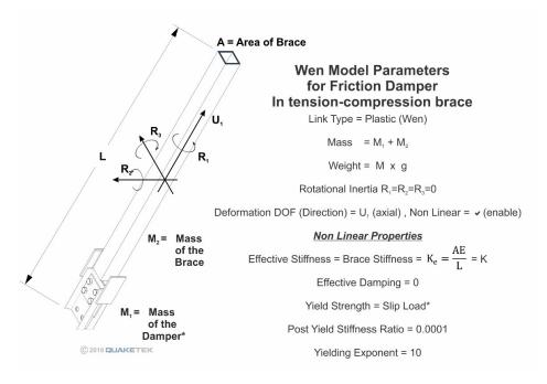
Figure 2-6 Wen Model parameters for Friction Dampers in tension-compression braces
