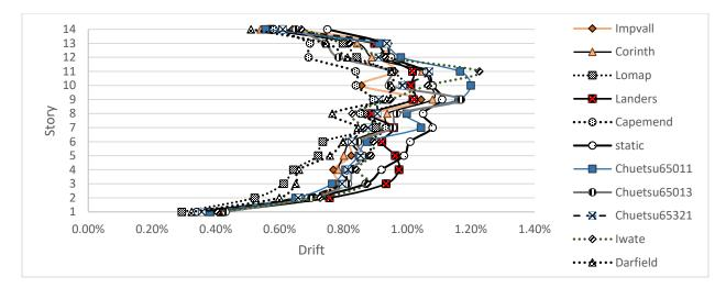
Figure 4-12 Time History drift for elastic with dampers model (EL-D)
