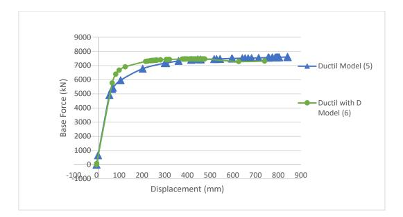
Figure 4-9 Pushover curve for ductile buildings (DUC) & (DUC-D)
