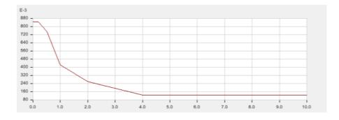
Figure 2-11 Vancouver Response Spectrum curve extracted from ETABS
