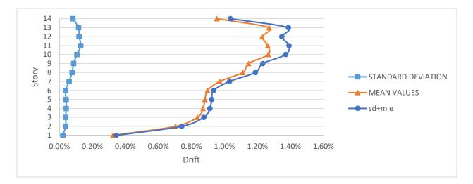
Figure 4-11 Standard deviation, mean values and sum for the Time History drift for elastic model (EL)
