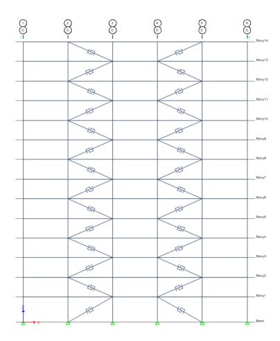
Figure 2-4 Frames views with dampers position
