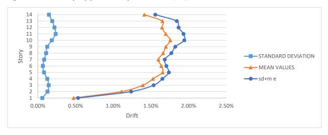
Figure 4-16 Standard deviation, mean values and sum for the Time History drift for moderately-ductile model (MD)
