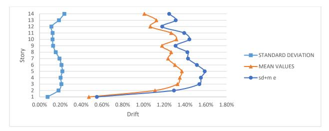
Figure 4-18 Standard deviation, mean values and sum for the Time History drift for moderately-ductile model with dampers (MD-D)
