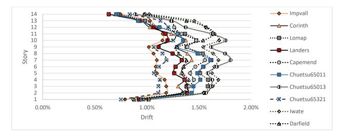
Figure 4-15 Time History drift for moderately- ductile model (MD)
