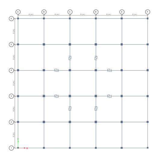
Figure 2-3 plans view with dampers
