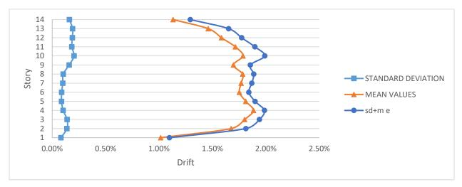
Figure 4-21 Standard deviation, mean values and sum for the Time History drift for ductile model (DUC)
