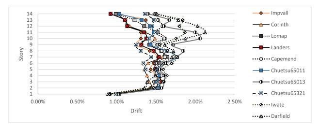
Figure 4-22 Time History drift for ductile model with dampers (DUC-D)
