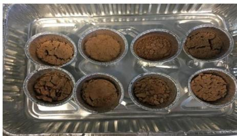
Figure 0-7 Sludge samples dried in oven at 105°C
