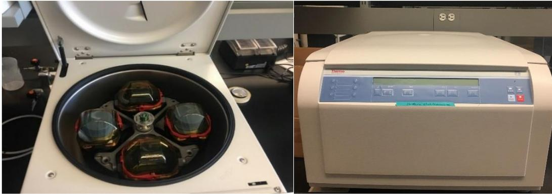
Figure 0-4 Centrifuge Thermo Scientific Sorvall ST 40 for 1-liter test
