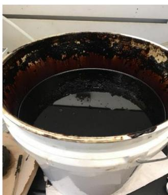
*Figure 0-2 Oily sludge sample stored in a 20 L bucket*
