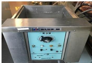
*Figure 0-10 Adjusting the temperature of centrifuge tubes using bath for oily sludge samples with Blue M Magni-Whirl1 MW-1120A-1 water bath*
