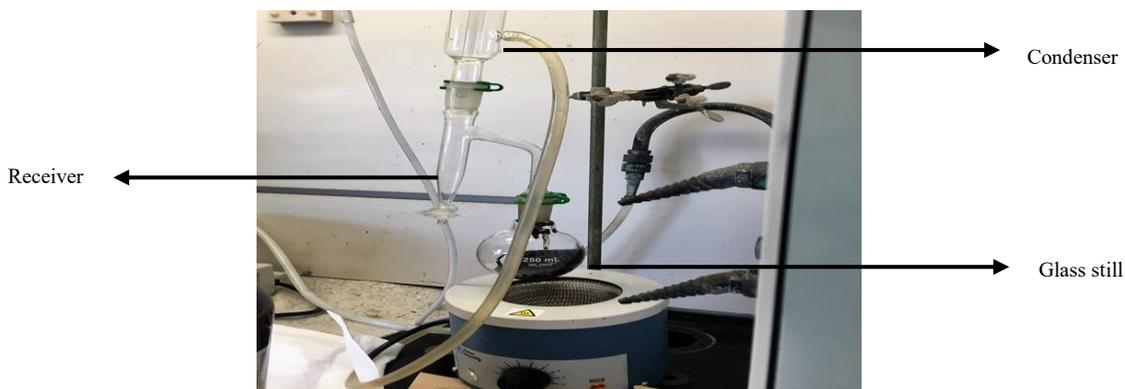
Figure 0-6 Typical assemblies for measuring water content by solvent extraction method (ASTM D95)
