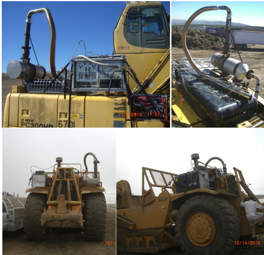
Figure 9 Field measurement of in-use activity (Tu 2011)
