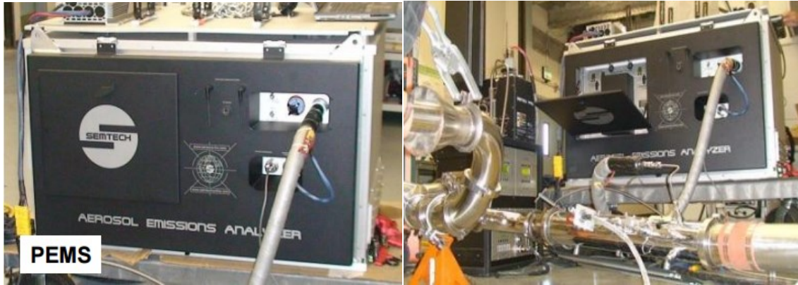
Figure 8 Portable emissions measurement system (Tu 2011)
