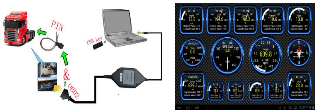
Figure 3-8: OBD II scanning system and sample outputs dashboard
