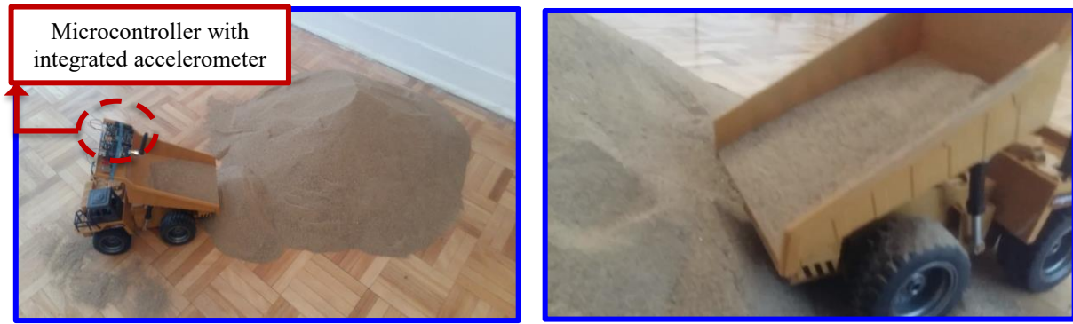
Figure 3-24: Acceleration recording for a scaled truck during dumping
