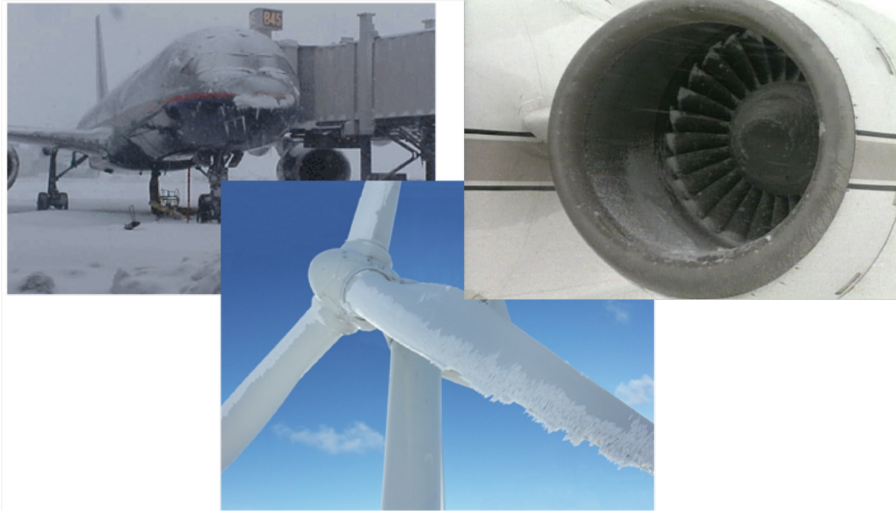
Figure 1.1: Ice accumulation on critical parts of airplane and wind turbines
