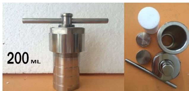
Figure 3.6. Pressurized autoclave, the capacity of the Teflon-lined autoclave: 200 ml.
