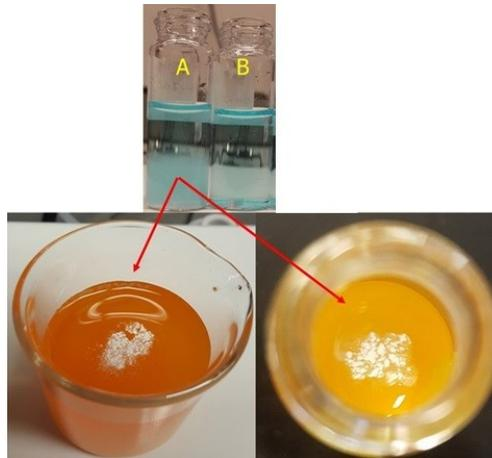
Figure 4.16. Relative water dispersibility of (A) Zn(OH)F and (B) ZnO.
