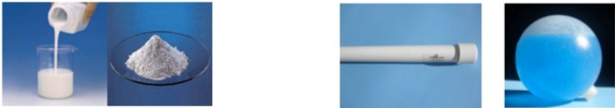
Figure 2-1. Micro-encapsulation and macro-encapsulation of PCM [14].
