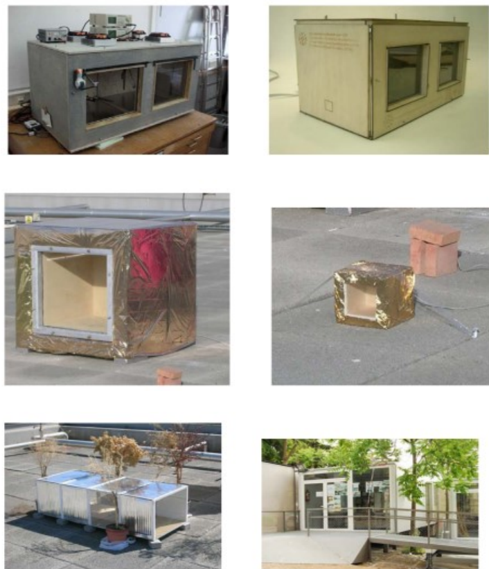
Figure 2-12. Sub-scale experiments with building glazing [23].
