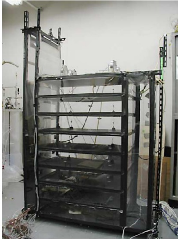
Figure 2-9. Solar chimney tests in a sub-scale eight-story building [21].
