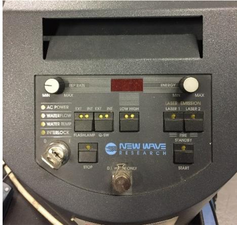
Figure A1-2 Control panel of laser
