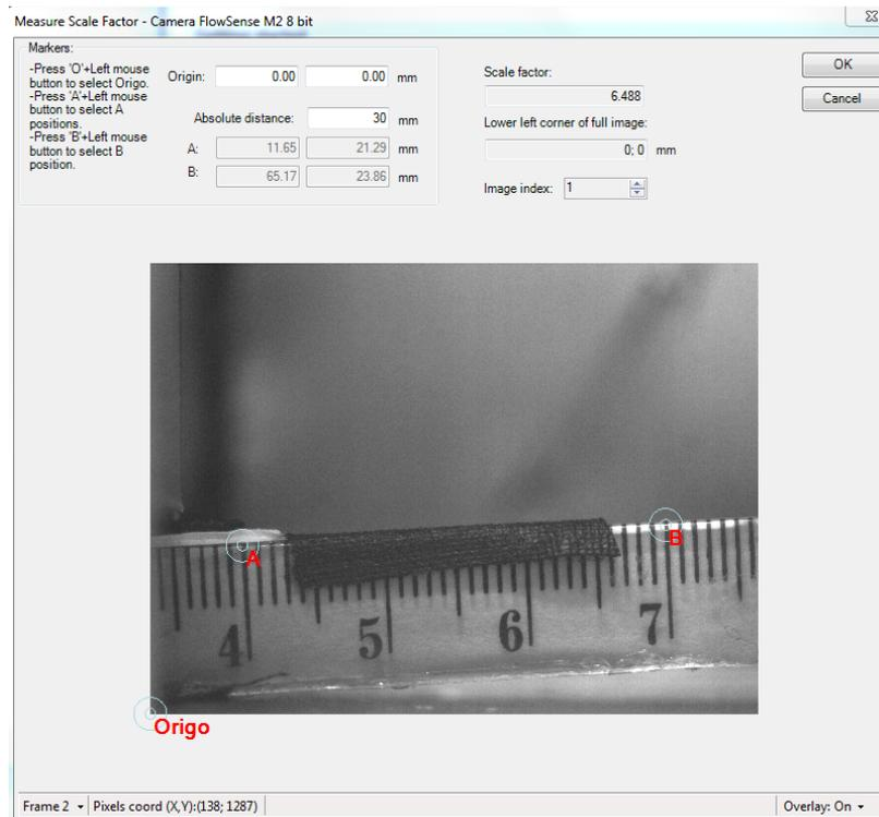
Figure A1-4 Measure scale factor for calibration
