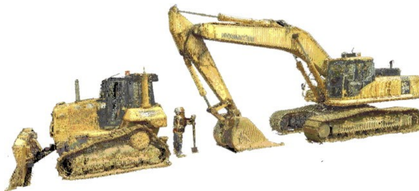
Figure 2-2 Hazardous situation of worker and equipment measured using a 3D laser scanner (Teizer et al. 2010)
