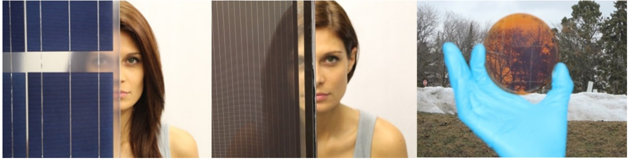
Figure 2.6: Summary of different types of STPV technologies. Left: Matrix-based semi-transparency, centre: Process-induced semi-transparency, right: Intrinsic semi-transparency. Taken with permission from [5]
