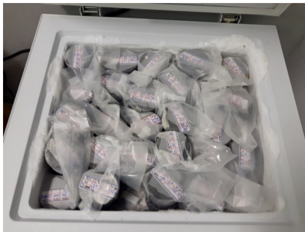
Figure 3. 18 Samples freezing and storage into a top opening freezer at -40\text{ }^{\circ}\text{C} .
