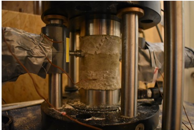
Figure 5. 1 Set-up of UCS test used at BEPL Laboratory.
