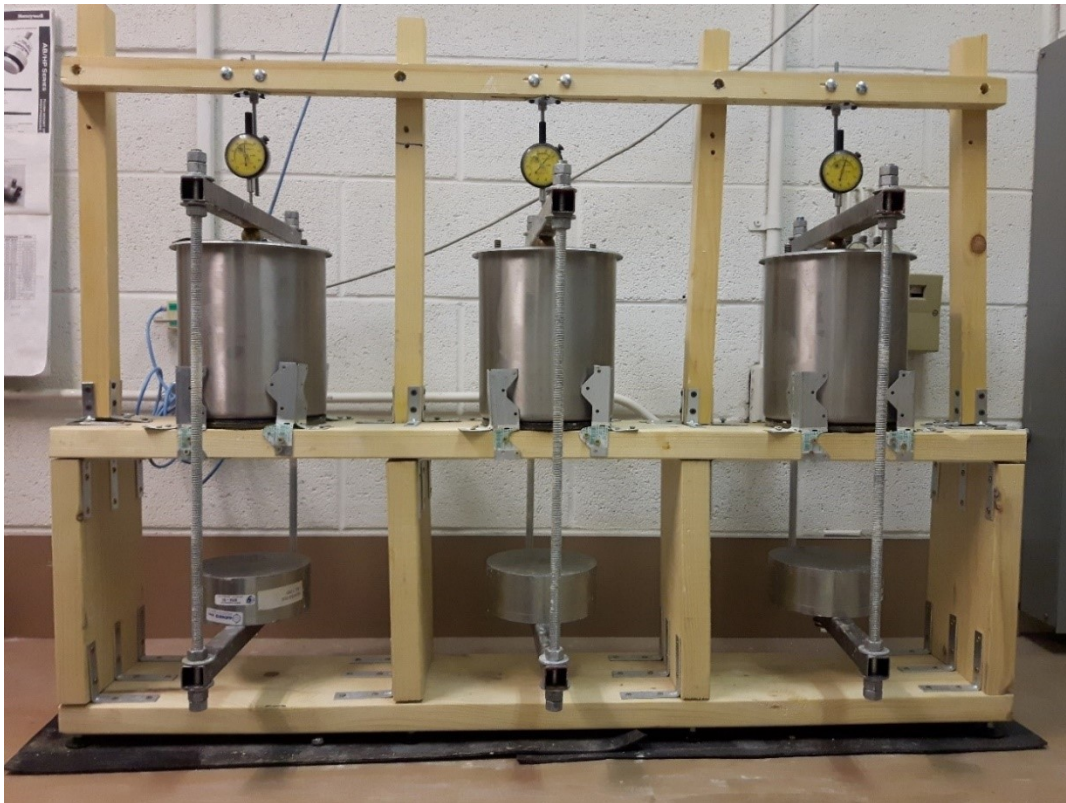
Figure 3. 9 The consolidation set-up.
