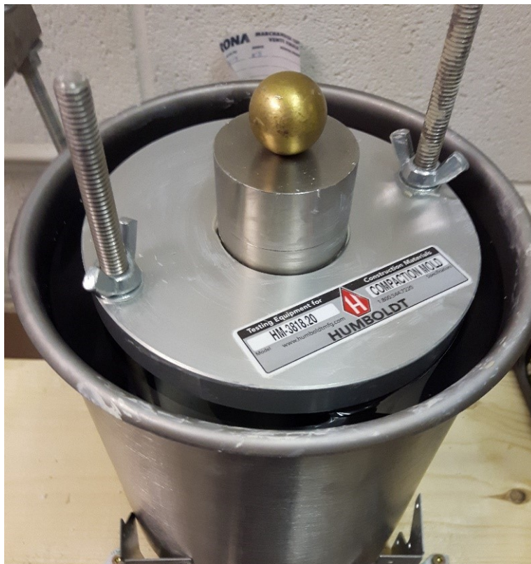
Figure 3. 6 The consolidation cell.
