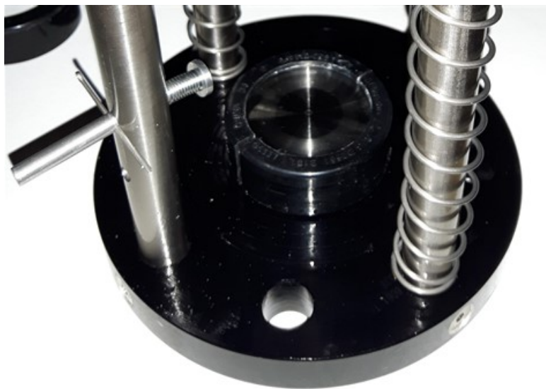
Figure 5. 3 Holders used for positioning frozen samples before the UCS test.
