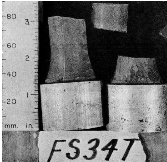
Figure 2. 8 Failure plane of tensile test for frozen silt samples (Haynes, 1978).
