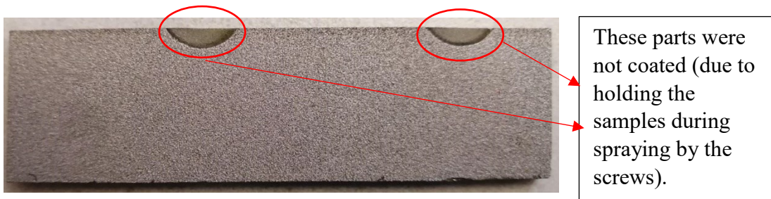
Figure 2.7: a grit-blasted 200 mesh sample after coating.
