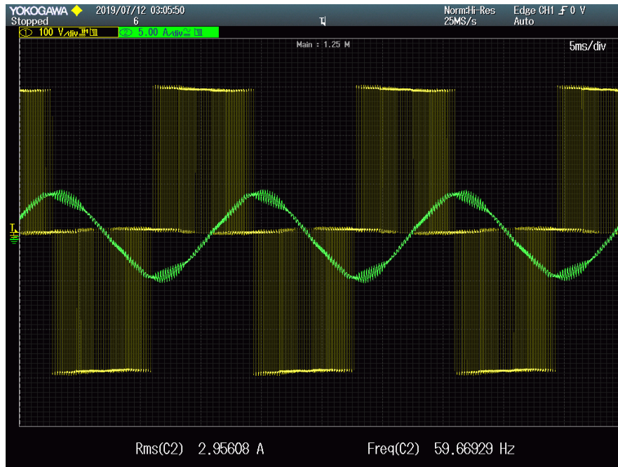
Figure 3.19: Line voltage V_{AB} and current I_A with the motor operating at 60 Hz.
