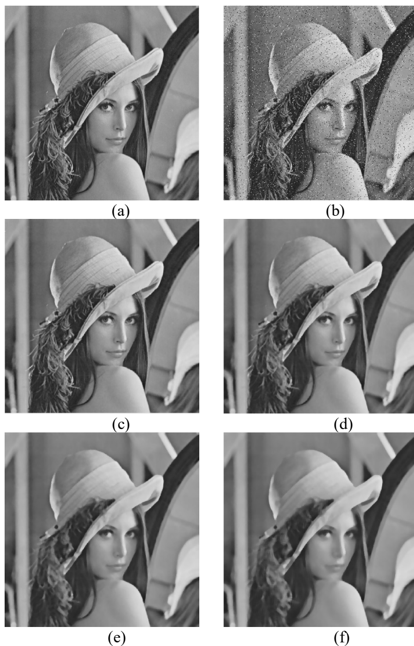
Figure 2.5 (a) Original Image (b) Image with 5% noise density (c-f) Images filtered using CMF with W_s = 3, 5, 7 and 9 , respectively.
