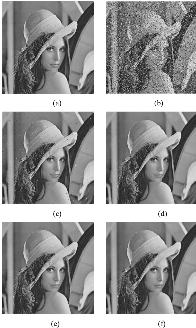
Figure 2.7 (a) Original Image. (b) Image with 25% noise density. (c-f) Images filtered using ASMF with W_s = 3, 5, 7 and 9 , respectively.
