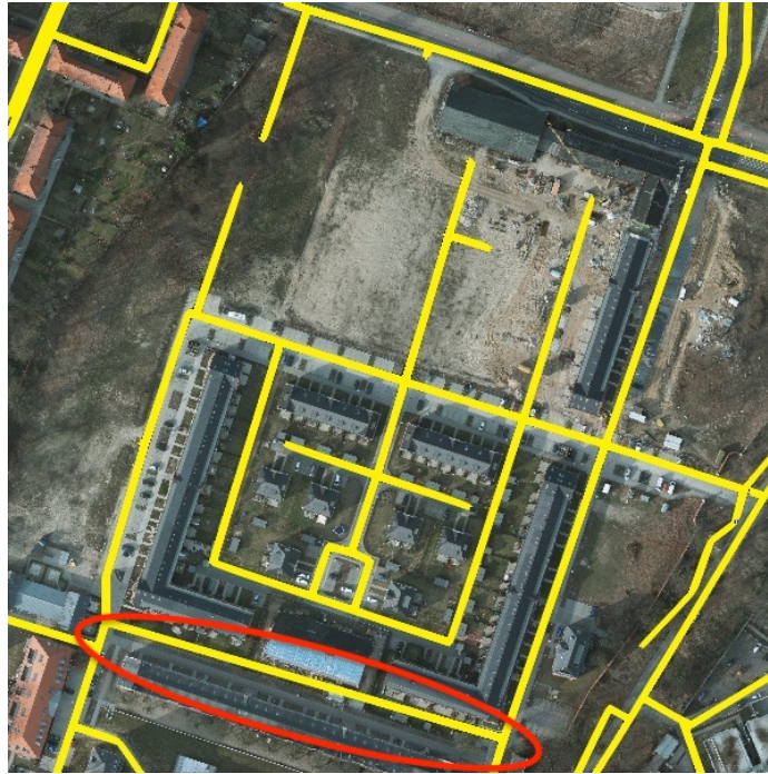
Figure 3.7: Example shows OSM data mistakes. Yellow lines are road data extracted from OpenStreetMap database. It is clear to see that in the region of the red circle, the entire road is misaligned with the actual one.
