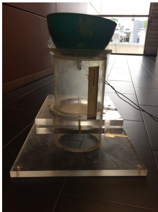
Figure 3-5 Photo of the filtration unit
