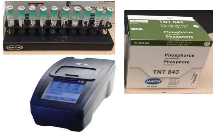
Figure 3-9 HACH test kit and spectrophotometer used for analyzing TP and DP
