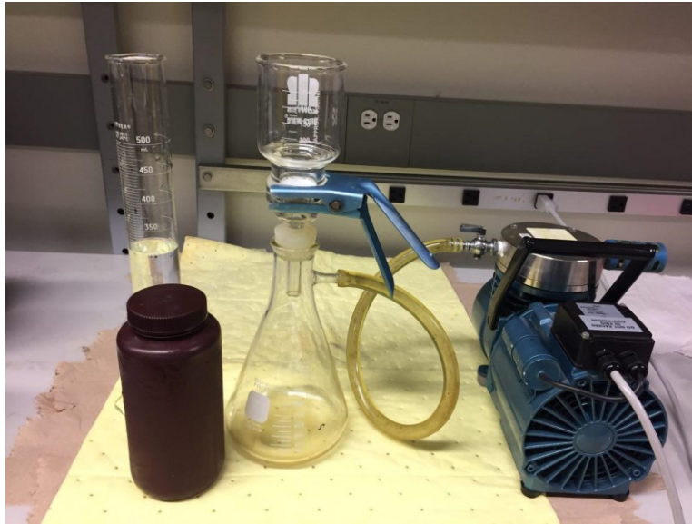
Figure 3-8 Separation of suspended solids using vacuum filtration system
