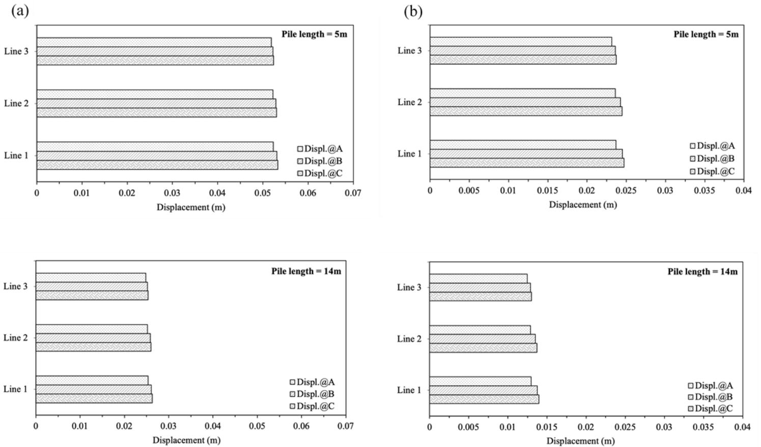
Figure 4.25 Vertical displacement in pile cap in 16-pile foundation: (a) medium sand soil, (b) dense sand soil.
