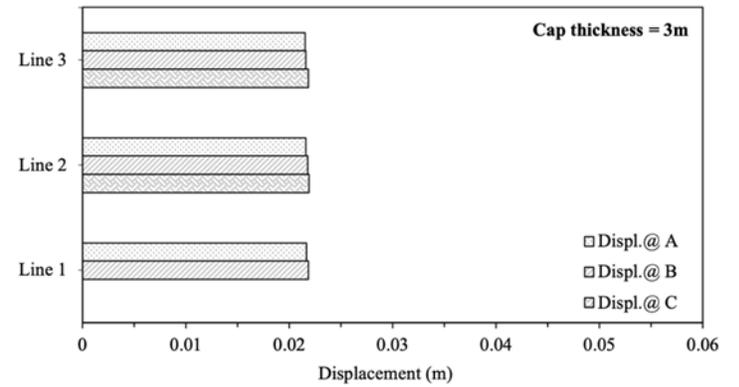
Figure 4.6 Vertical displacement in pile cap in 16-pile foundation in medium sand soil.
