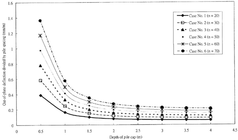
Figure 2.2 Curvature versus depth of the cap for variable number of floors (Cheng, 2005).
