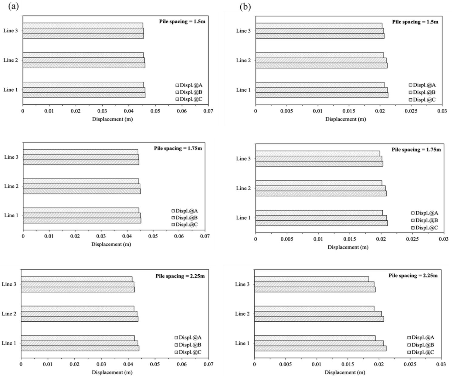
Figure 4.16 Vertical displacement in pile cap in 9-pile foundation: (a) medium sand soil, (b) dense sand soil.
