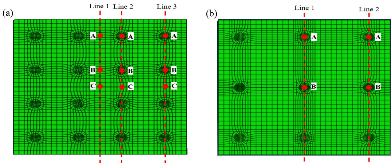
Figure 4.5 Location of typical points to examine the displacement: (a) 16-pile foundation, (b) 9-pile foundation.
