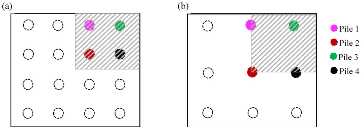
Figure 4.1 Layout of piles under examination: (a) 16-pile foundation, (b) 9-pile foundation.
