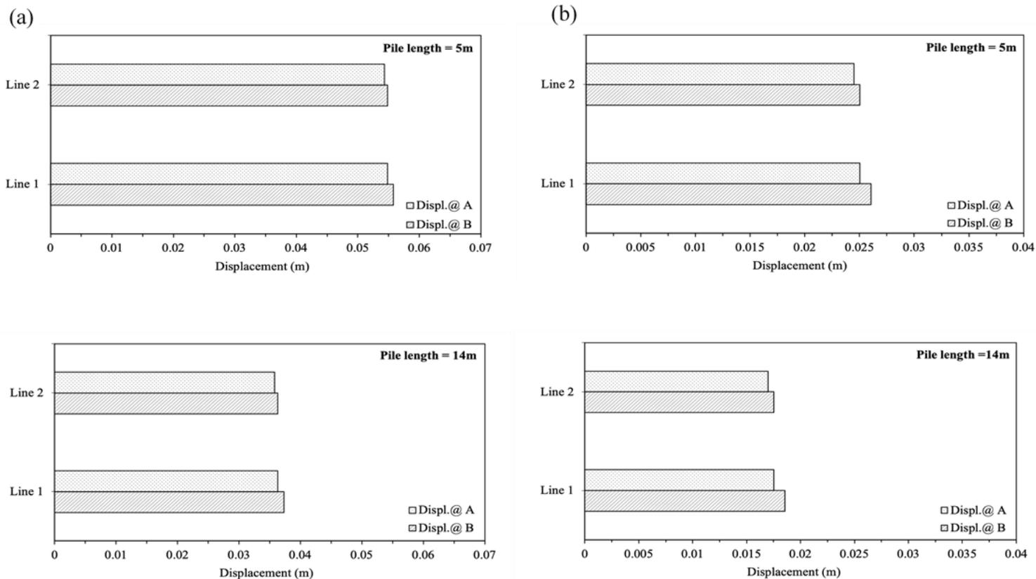
Figure 4.26 Vertical displacement in pile cap in 9-pile foundation: (a) medium sand soil, (b) dense sand soil.
