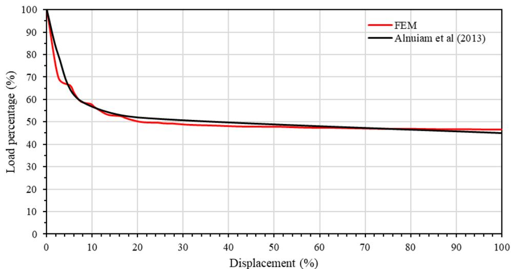
Figure 3.9 Comparison of the results of load sharing percentage vs pile cap displacement.
