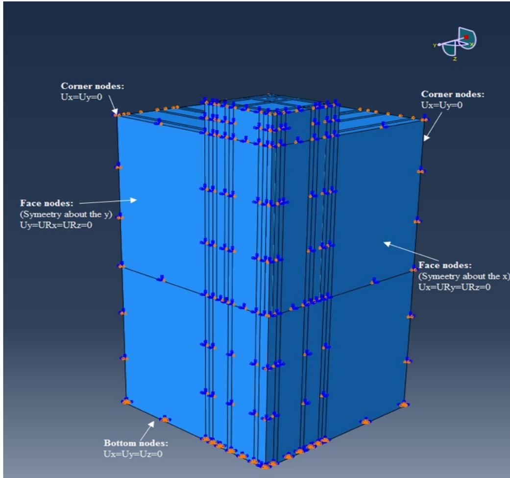
Figure 3.6 Boundary conditions defined in the model.
