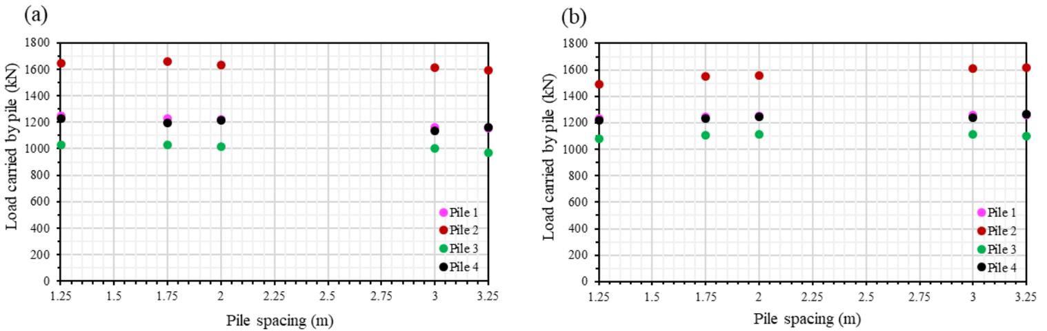
Figure 4.13 Pile load vs pile spacing for the 9-pile foundation: (a) medium sand soil, (b) dense sand soil.
