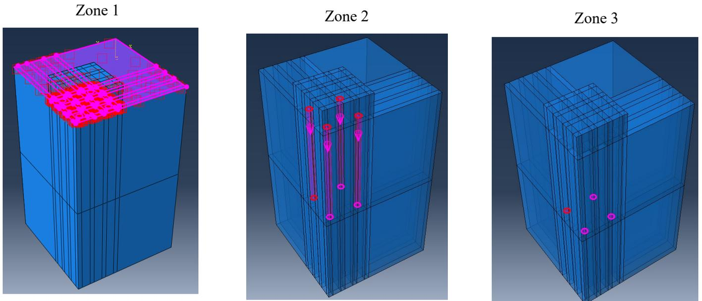
Figure 3.4 Contact zones defined in ABAQUS.
