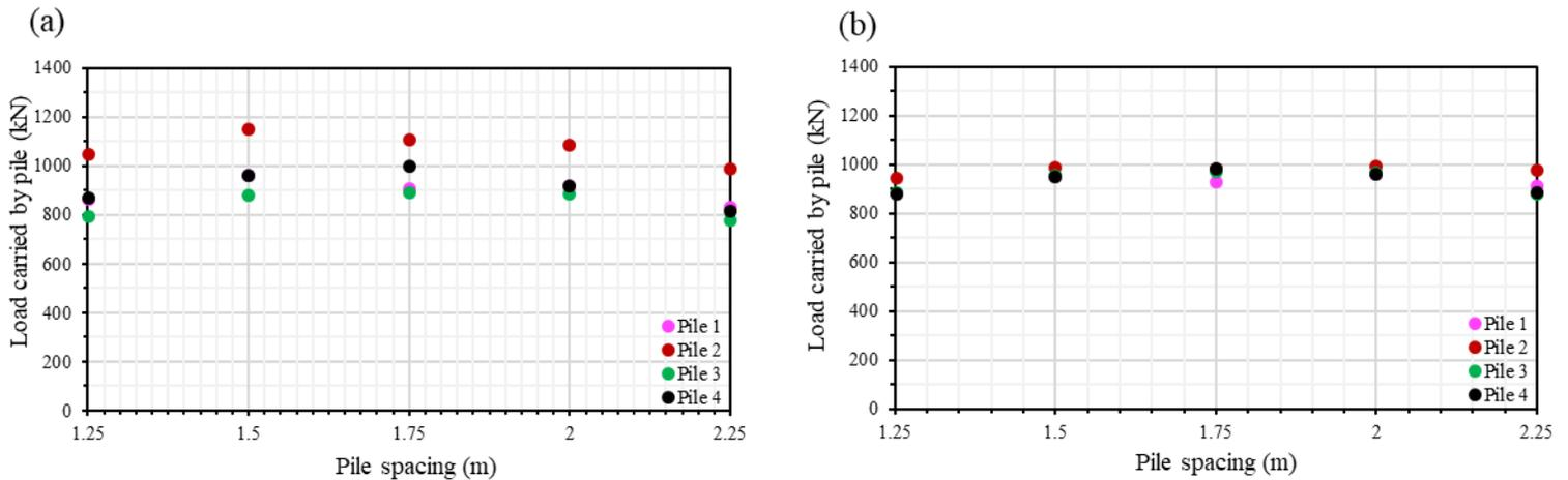
Figure 4.12 Pile load vs pile spacing for the 16-pile foundation: (a) medium sand soil, (b) dense sand soil.
