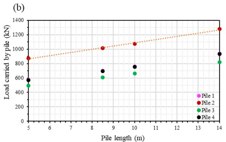
Figure 4.23 Pile load vs pile length for the 9-pile foundation: (a) medium sand soil, (b) dense sand soil.
