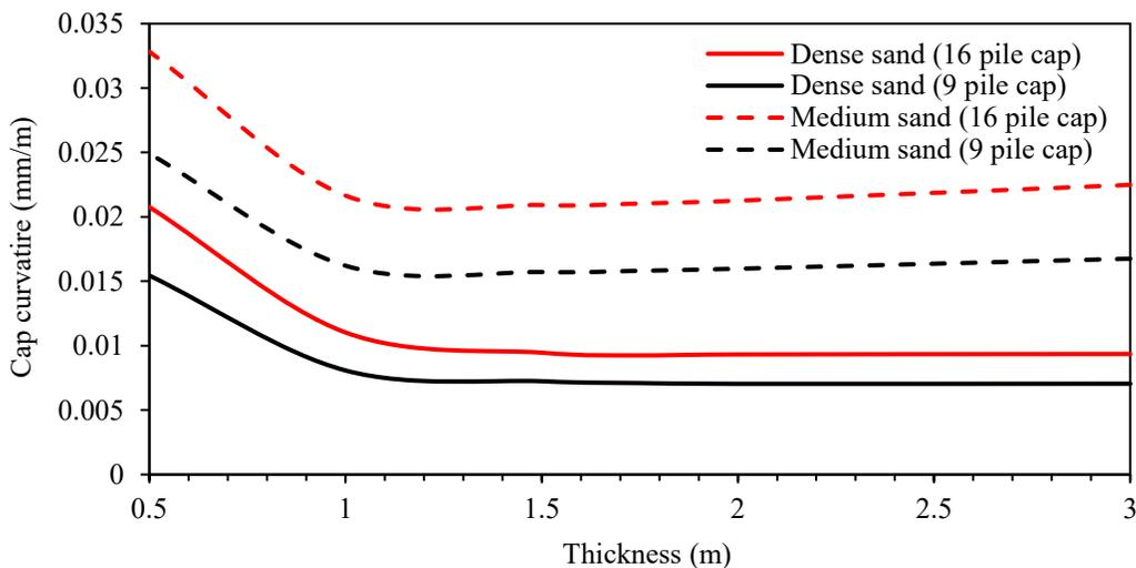
Figure 4.10 Curvature *vs* cap thickness for 9- and 16-pile foundation.
