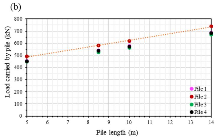
Figure 4.22 Pile load vs pile length for the 16-pile foundation: (a) medium sand soil, (b) dense sand soil.
