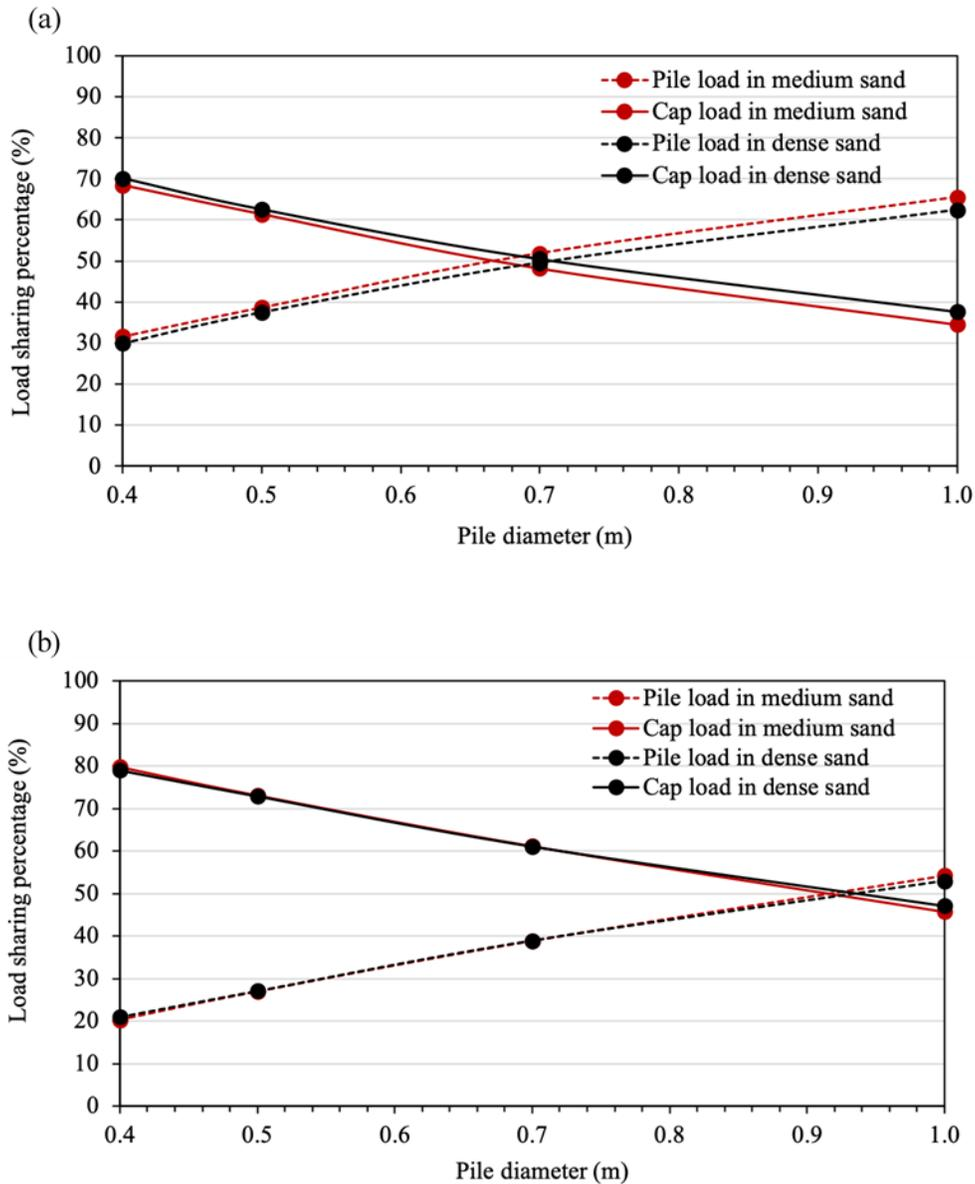
Figure 4.19 Percentage of load sharing vs pile diameter: (a) 16-pile foundation, (b) 9-pile foundation.
