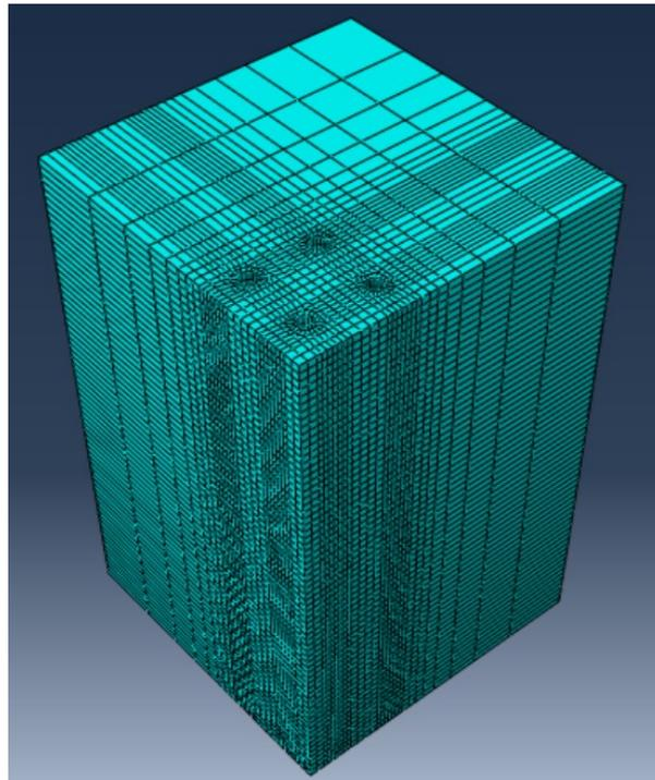
Figure 3.3 ABAQUS ¼ model for the soil in 16-pile foundation.
