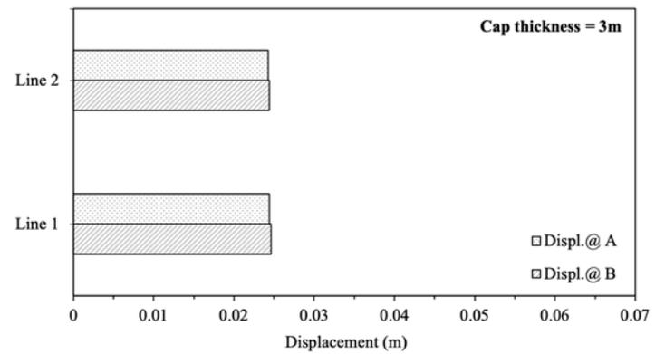
Figure 4.9 Vertical displacement in pile cap in 9-pile foundation in medium sand soil.
