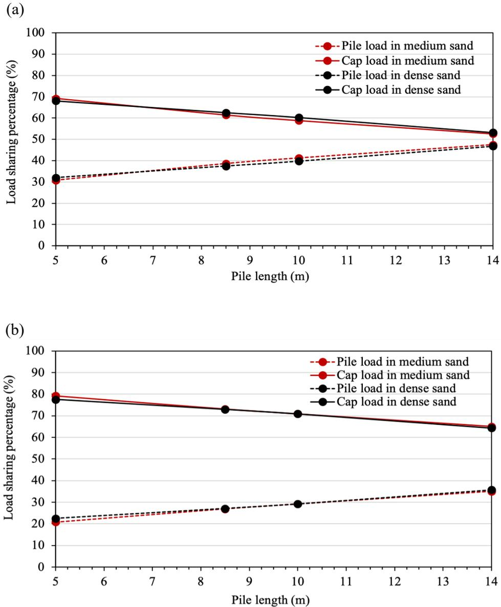
Figure 4.24 Percentage of load sharing vs pile length: (a) 16-pile foundation, (b) 9-pile foundation.
