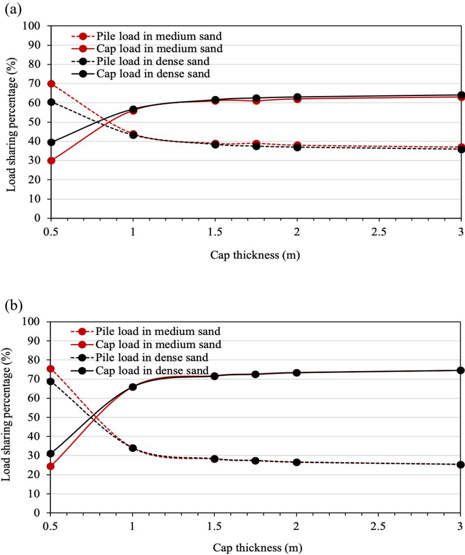
Figure 4.4 Percentage of load sharing vs pile cap thickness: (a) 16-pile foundation, (b) 9-pile foundation.
