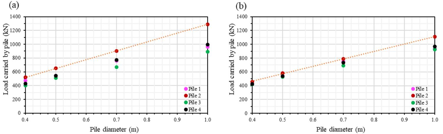
Figure 4.17 Pile load vs pile diameter for the 16-pile foundation: (a) medium sand soil, (b) dense sand soil.
