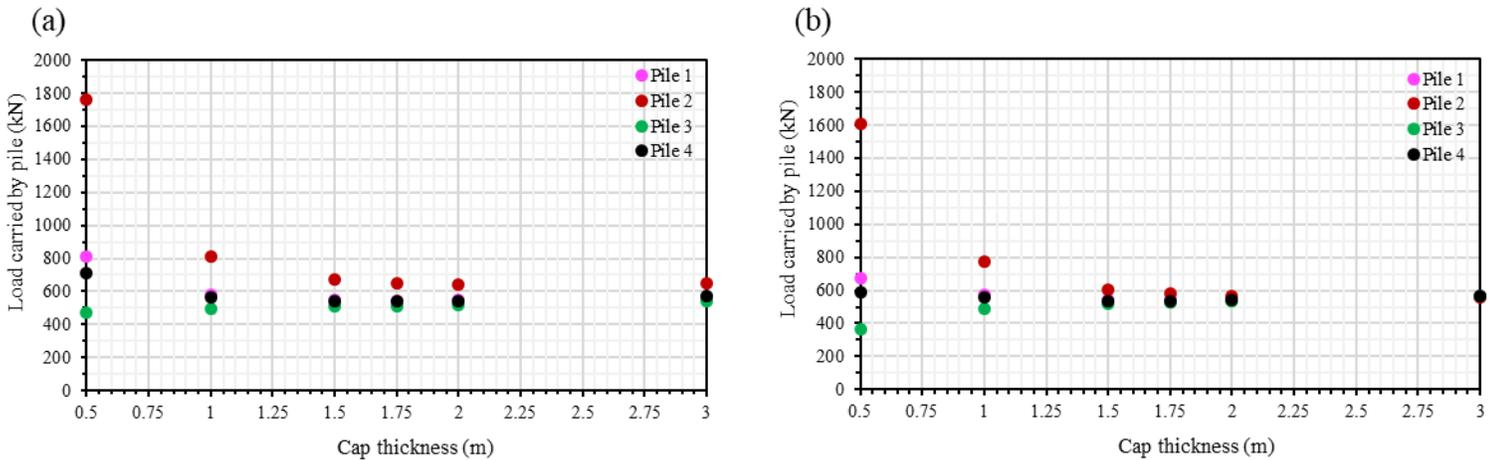
Figure 4.2 Pile Load vs pile cap thickness for the 16-pile foundation: (a) medium sand soil, (b) dense sand soil.
