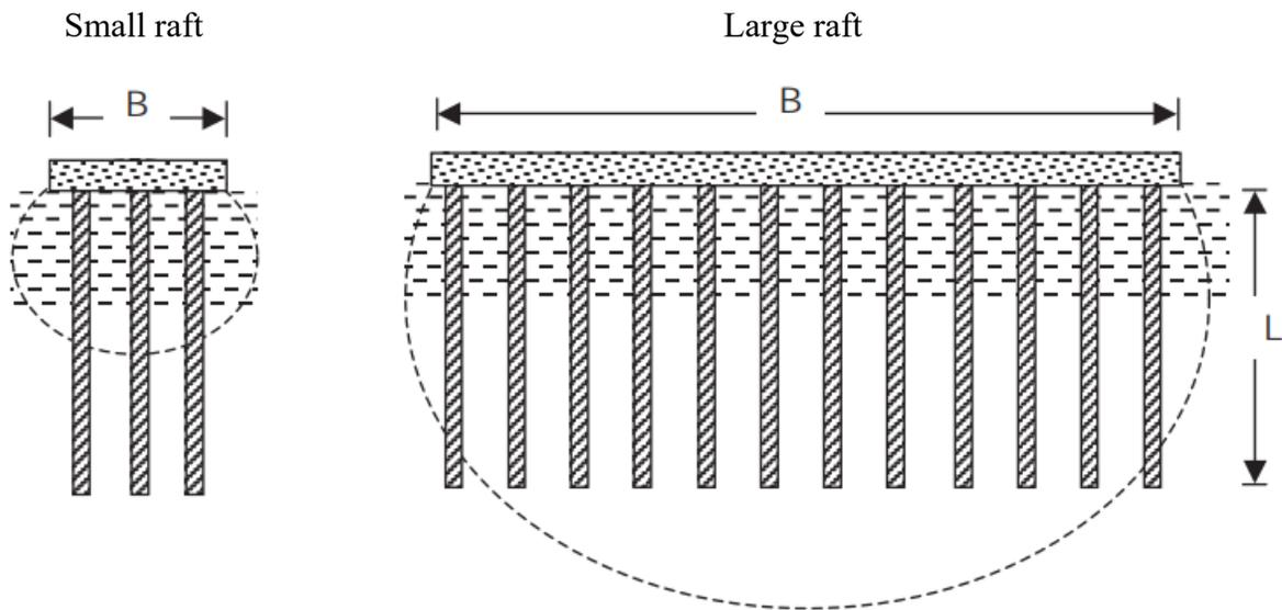
Figure 2.1 Illustration of small and large pile rafts adapted from Viggiani et al. (2012).
