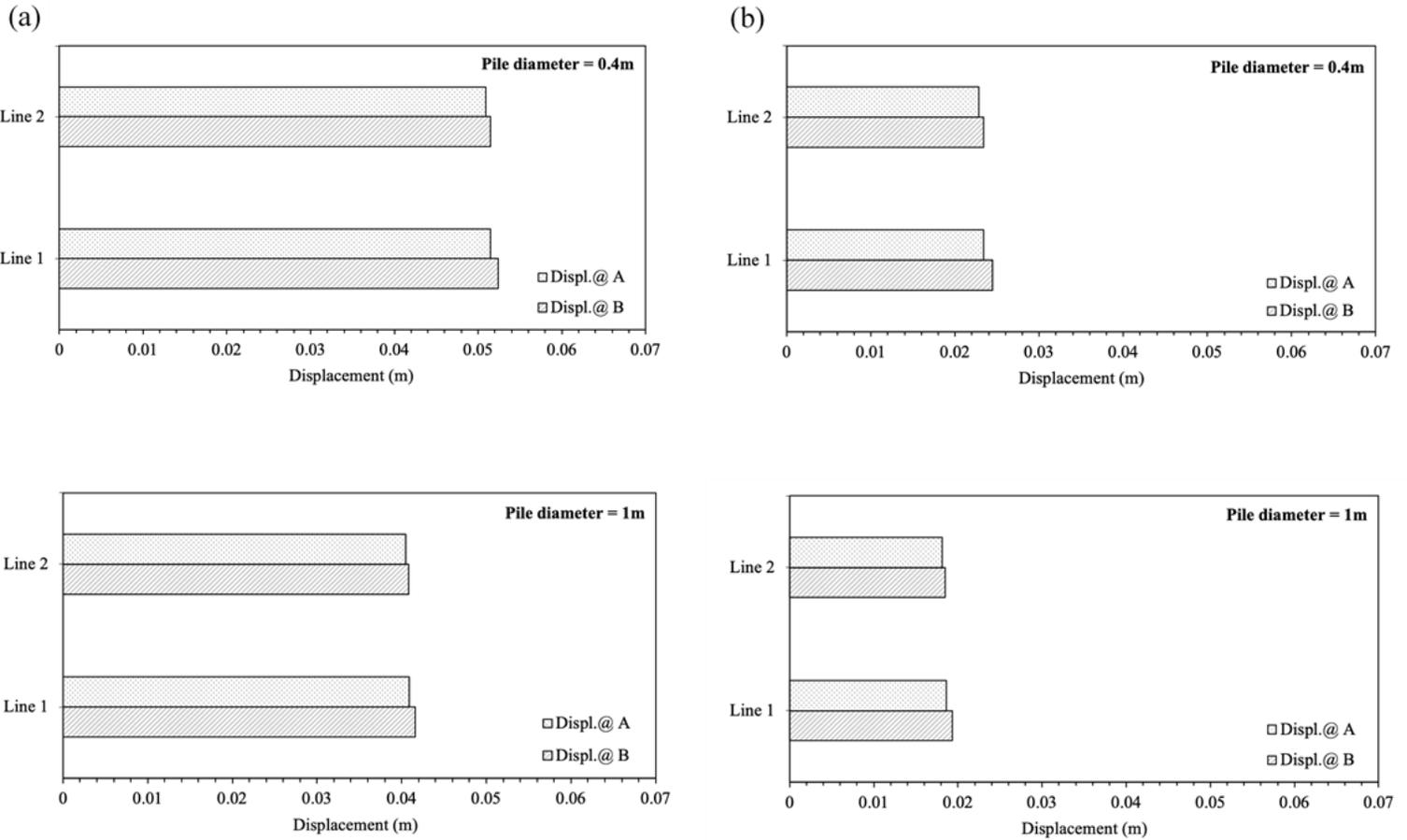
Figure 4.21 Vertical displacement in pile cap in 9-pile foundation: (a) medium sand soil, (b) dense sand soil.
