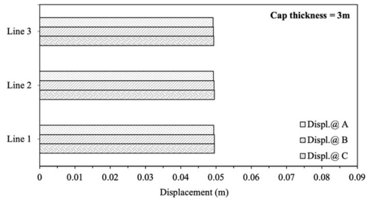
Figure 4.7 Vertical displacement in pile cap in 16-pile foundation in dense sand soil.
