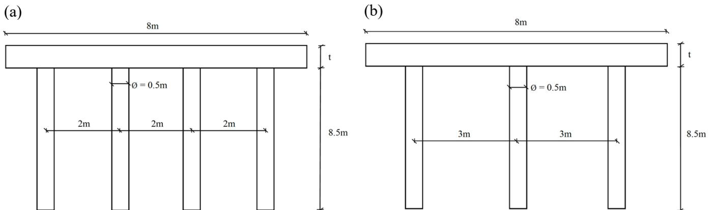
Figure 3.1 Elevation view of the foundations: (a) 16-pile foundation, (b) 9-pile foundation.
