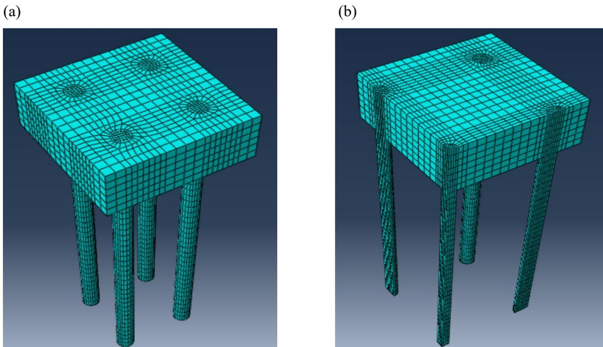
Figure 3.2 ABAQUS  $\frac{1}{4}$  model: (a) 16-pile foundation, (b) 9-pile foundation.
