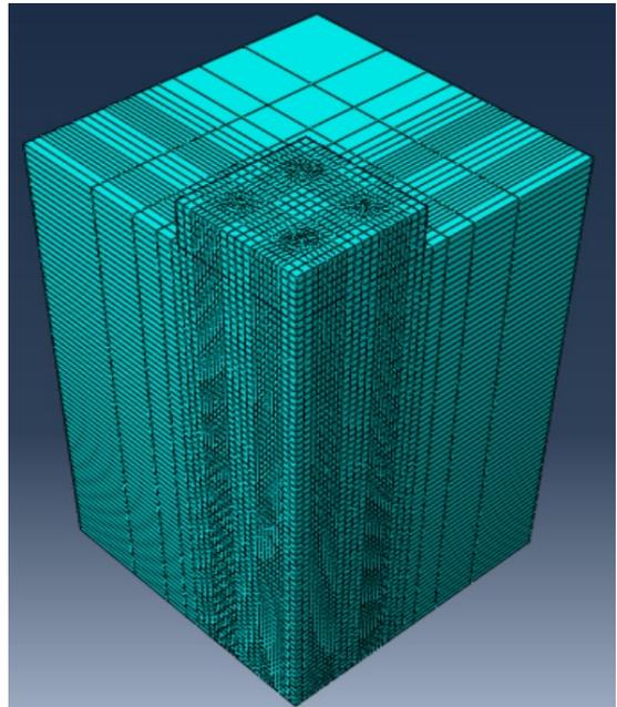
Figure 3.5 ABAQUS meshing for  $\frac{1}{4}$  of the 16-pile foundation: (a) partitions assigned, (b) final meshed model.
