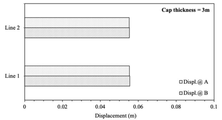
Figure 4.8 Vertical displacement in pile cap in 9-pile foundation in medium sand soil.
