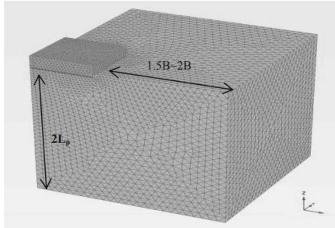
Figure 3.7 Finite element model as Alnuiam et al. (2013).
