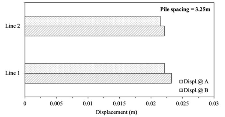
Figure 4.15 Vertical displacement in pile cap in 16-pile foundation: (a) medium sand soil, (b) dense sand soil.
