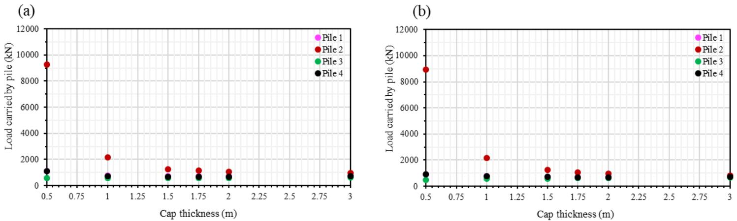
Figure 4.3 Pile load vs pile cap thickness for the 9-pile foundation: (a) medium sand soil, (b) dense sand soil.
