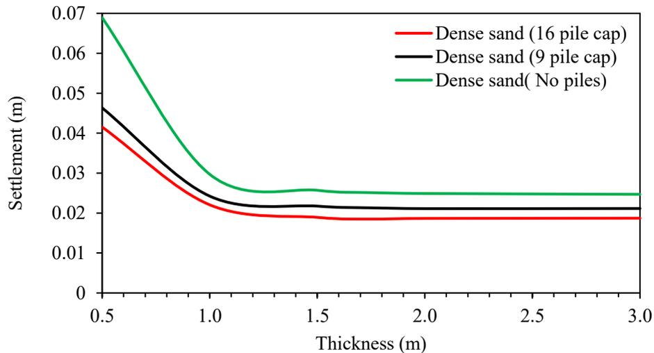
Figure 4.11 Center settlement of the pile cap foundation with variable cap thicknesses for different pile cap foundations.
