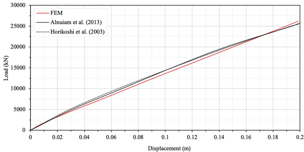
Figure 3.8 Comparison of the results of pile cap displacement vs axial loading.
