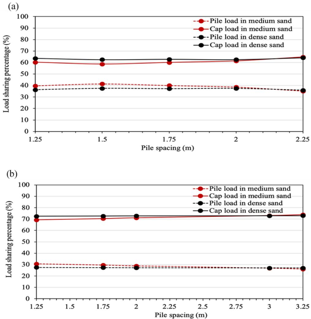
Figure 4.14 Percentage of load sharing vs pile spacing: (a) 16-pile foundation, (b) 9-pile foundation
