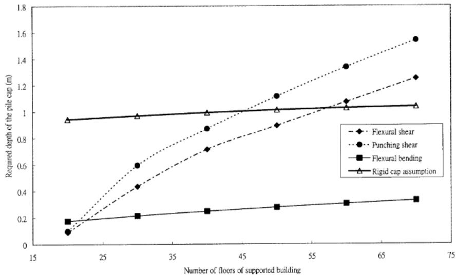
Figure 2.3 Comparison of the design depth of a pile ap with different methods (Cheng, 2005).
