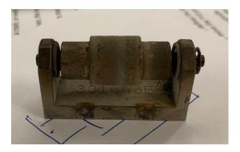
Figure 21. Consolidation roller of AFP setup
