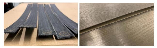
Figure 7. Distortion of the composite laminate during and after the process
