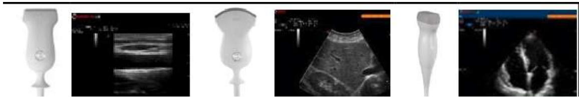
Figure 1.3: From left to right: linear, curvilinear and phased-array ultrasound probes and images collected by them. Picture courtesy of Luca et al., 2018.
