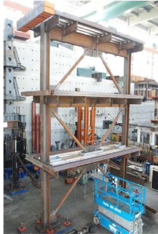
Figure 2.11 Test specimen TCBF2-HSS at NCREE in Taipei, Taiwan (Lumpkin, 2009)
