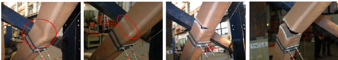
Figure 2.13 North brace of Specimen TCBF1-HSS on the 1 st storey a) Brace fracture at plastic hinge b) Initial tear lines c) Partial fracture d) Fracture Opening (Lumpkin, 2009)
