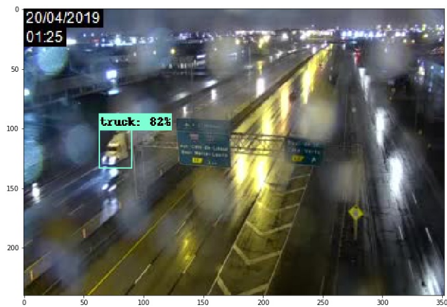
Figure 32: An Example of the Object Detection Model Output on Images with Trucks In Them
