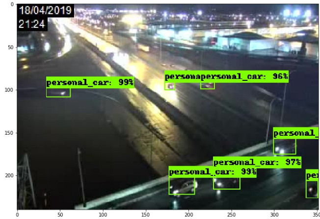
Figure 30: An Example of the Object Detection Model Output on Images with Complex Road Architecture and Low Light Setting
