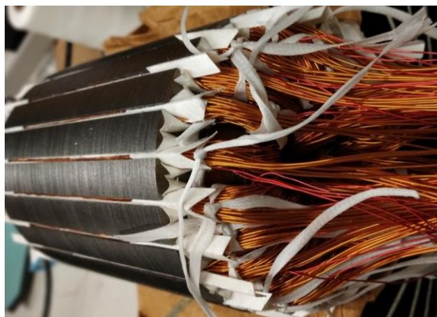
Figure 3.3: The excitation coil during winding process
