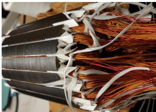
Figure 3.3: The excitation coil during winding process
