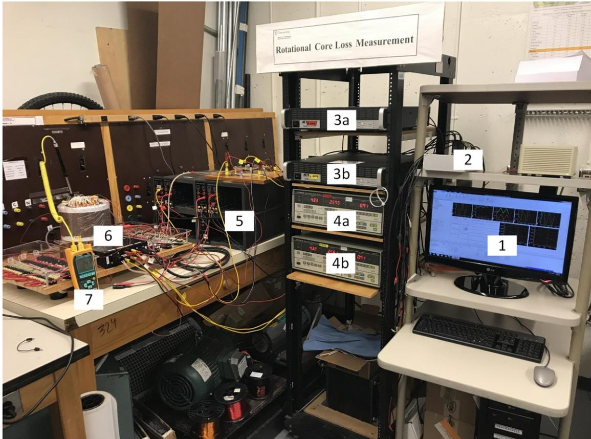
Figure 3.15: The experimental setup (1) Computer (2) dSPACE® DS1103 controller (3) Power amplifier (4) Power meters (5) Voltage/current isolation (6) Tester setup with stator under test (7) Thermometer and thermocouples
