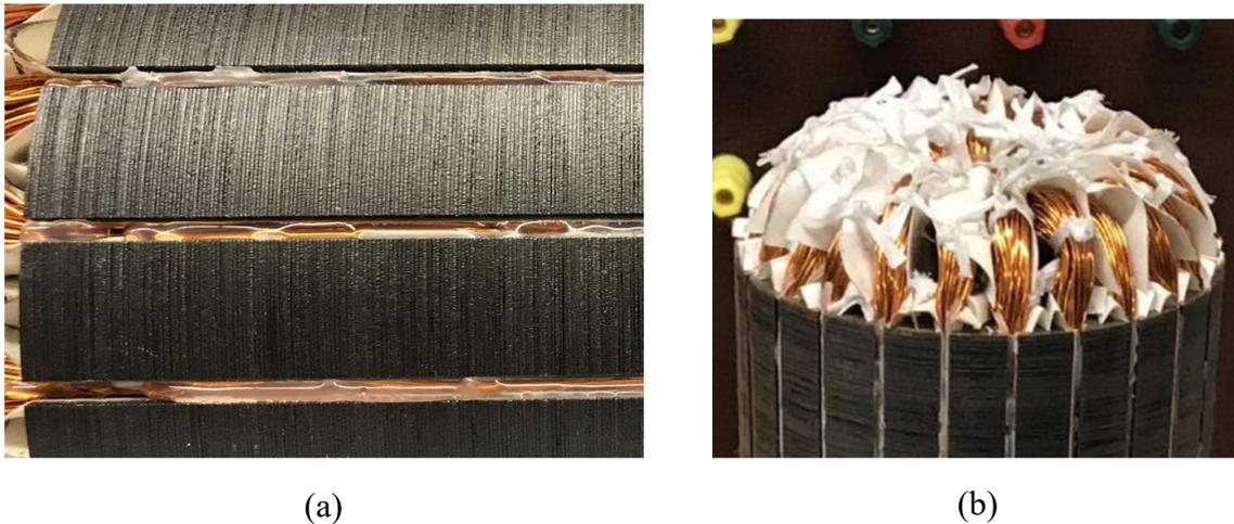
Figure 3.11: The tester with (a) Glue filled slots to insulate excitation coils from the top edge of the slots (b) Excitation coil end-connections separated from each other with insulation paper
