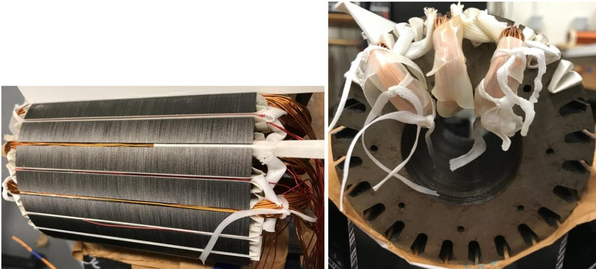
Figure 3.9: Tester windings during the winding process
