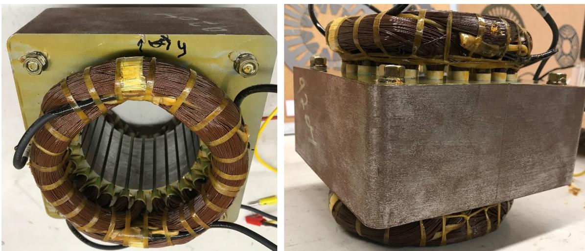
Figure 1.7: 24 Slots Induction Machine Round Single sheet tester
