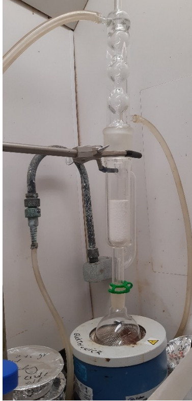
Figure 3-2 Water content measurement by solvent extraction method (ASTM D95-05,2005) in the lab
