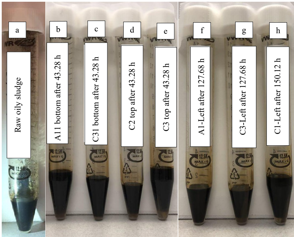
Figure 4-48 Samples after BS&W test: a) raw oily sludge; b) bottom extraction from A11 after 43.28 h; c) C31 bottom, 43.28 h; d) C2 top, 43.28 h; e) C3 top, 43.28 h; f) A1-Left top, 127.68 h; g) C3-Left top, 127.68 h; h) C1-Left top, 150.12 h
