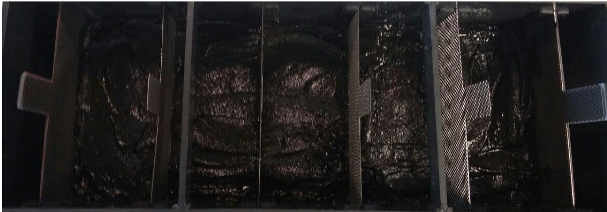
Figure 3-10 EK reactor after filling with the raw oily sludge
