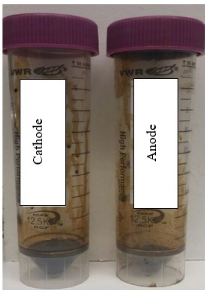
Figure 4-7 Qualitative assessment of Test S3 (voltage gradient of 2.05 V/cm, sample C mix (C1-C8))
