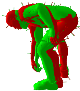
Figure 23: Figure demonstrating mesh based retargeting from the source character (green) to the target character (red) for a kneeling down motion.
