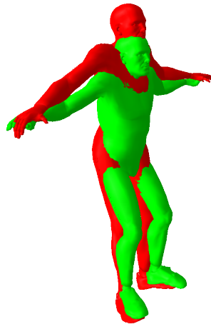
Figure 12: Two rigged meshes overlaid on each-other, with the animation from the green character being retargeted onto the red character.
