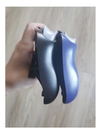
Figm · e VI2 shell backs of a GameCube controller. The black/ first one includes the spring resistance in the triggers, the second/purple shell has the springs removed. This is a common hardware mod for SSBM. This image shows the slight height difference for controller triggers. Many people only do this mod to one side. It is entirely player specific and subjective to a player's preferred controller feel.
