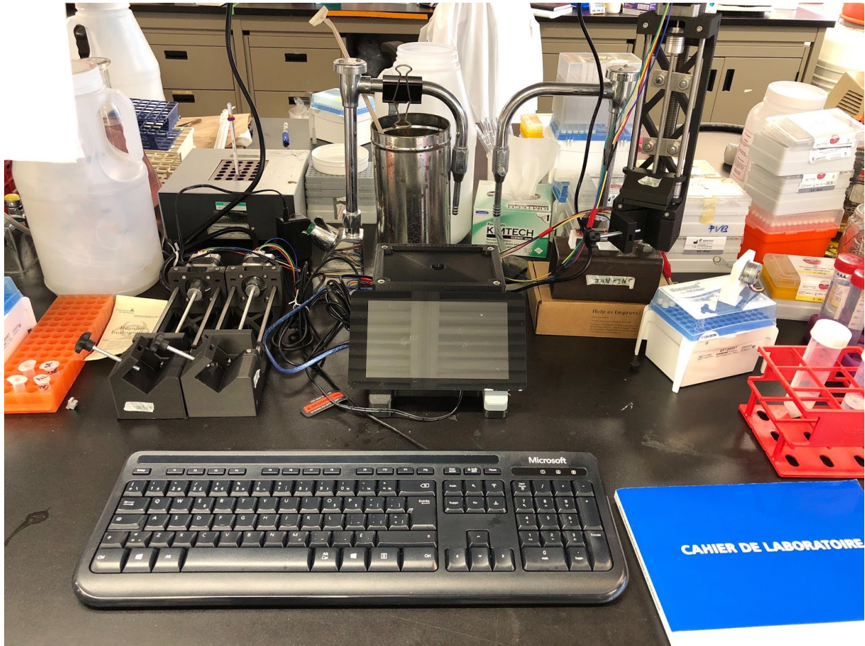
Supplemental Figure 10. Our fungal DROP-seq system. The small screen is driven by a Raspberry Pi CPU and controls the pumps: two on the left for oil and cells and one on the right (vertical) for beads. The microfluidic PDMS sits on the small black platform behind the screen.
