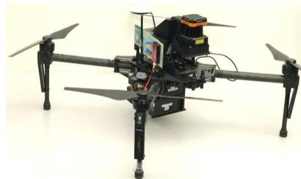
(b) Platform with vertical LiDAR
