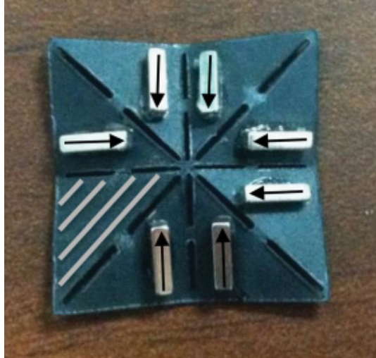
FIGURE 2.4: Polypropylene waterbomb samples were created with a laser cutter. Gray hatching indicates the ground panel. Permanent magnets with magnetization direction marked with black arrows were attached to each ungrounded panel to match the configuration determined from the dynamic model. © 2015 IEEE.
