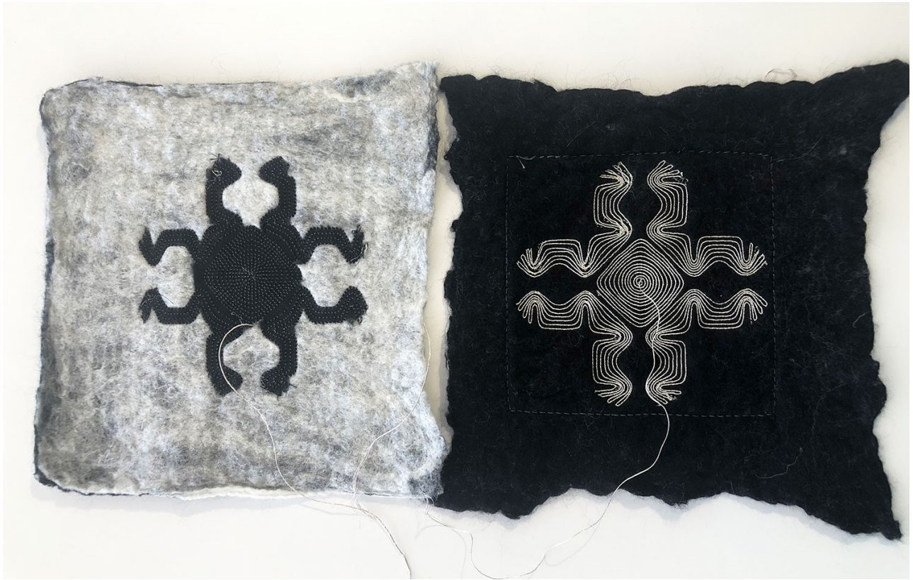
Figure 28 Symmetrical fabric speaker design and the test that offered the best overall result
