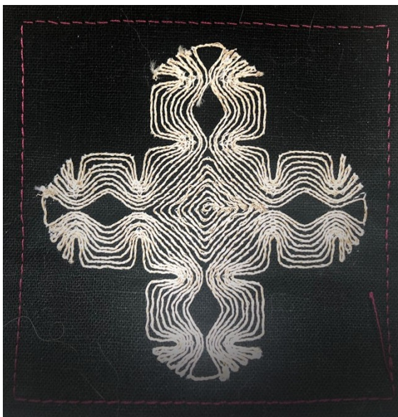
Figure 23 First phase of prototyping fabric speaker experiments (They did not produce sound)
