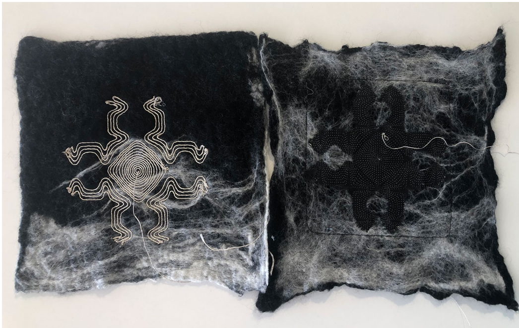
Figure 29 Symmetrical fabric speaker design and the test that offered the best overall result
