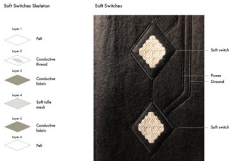
Figure 41 How are soft switches made? On the left: technical diagram of materials involved in a soft switch. On the right: final soft switches on the sonic felted garment
