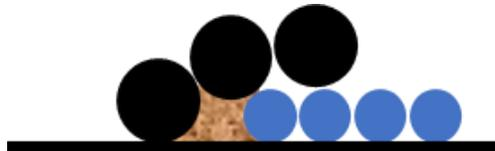
Figure 3-11: unfilled space (in brown) between two flattened particles in the flattened model
