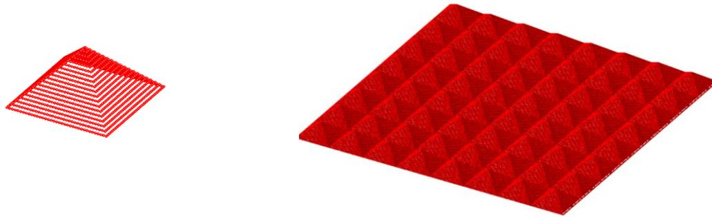
Figure 3-2: Substrate geometry simulated by cone shaped asperities
