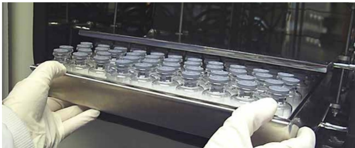
Fig. 2-7: A shelf with vials loaded inside the vacuum chamber
