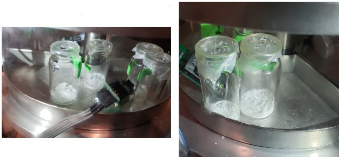
Fig. 5-58: Vials with sublimated material along with thermal sensors
