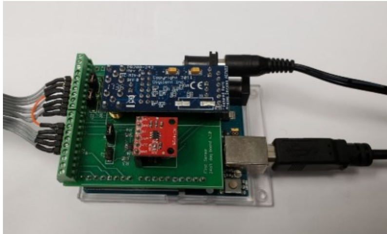
Fig. 5-32a: Data acquisition system
