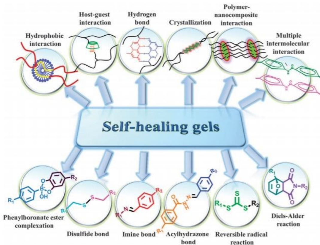
Figure 1.1 An illustration of typical reversible linkages reported in literature for the development of novel self-healable materials. 7
