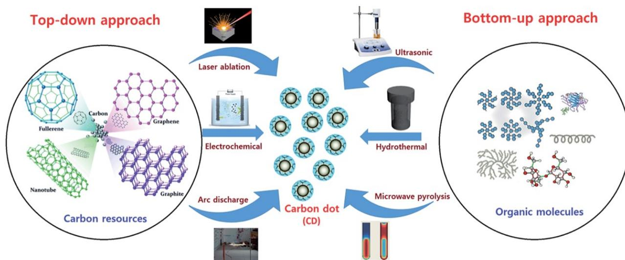
**Figure 8.** Top-down and bottom-up approaches for the synthesis of carbon dots (figure adapted from De *et al.*).<sup>66</sup>
