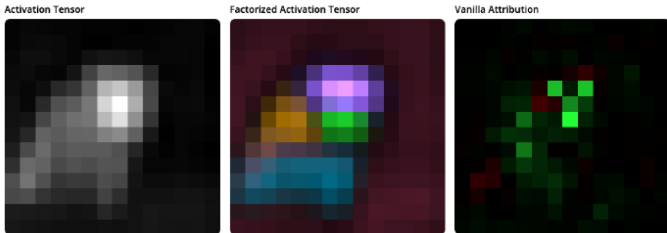
Figure 32: A snapshot of the Overview section, extended view panel. Left: sum-reduced activation tensor. Middle: latent spatial factors from NMF, overlaid. Right: vanilla attribution map.
