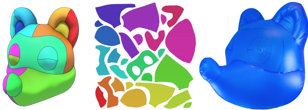
Figure 16: Inflatible Balloons. Framework to design inflatable balloons based on a shape objective.
