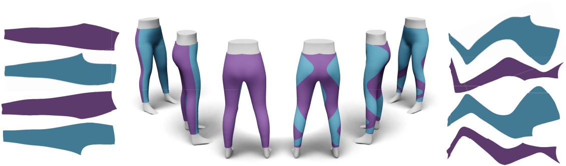
Figure 35: Pants stretched in the direction of the circumference of the legs. The image shows the initial cloth with its patterns (left) and its optimized version using the seam traction objective (right).
