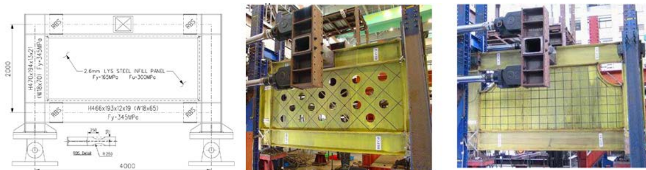
Figure 2.3: Vian and Bruneau (2004) test Specimens with solid panel (right), panel with 20 holes (center) and panel with cutout on the top corners (left)
