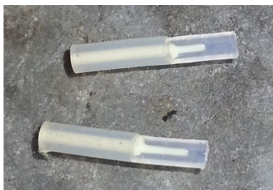
Figure 61 Image of fabricated 1/8" PTFE tubes after being cut and filled with PVA glue. The right-hand section with half of the tube removed was placed against the fishing line to act as a template for the conduits that joined the laminar flow channel to the BGE supply and waste tubing.
