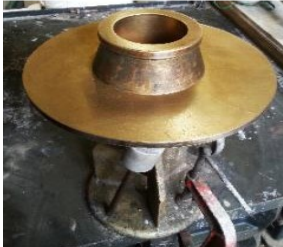
Figure 5-3 Flow table test for flowability evaluation
