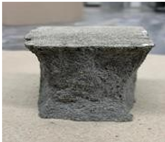
Figure 5-19 Cube failure shape after testing under compression load.
