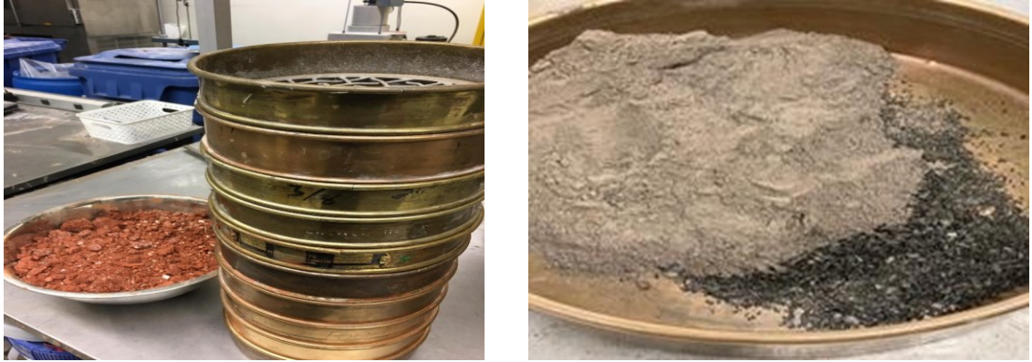
Figure 5-1 Sieve analysis test for red mud and PPFA
