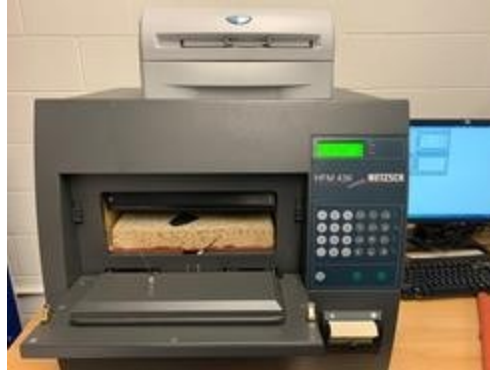
Figure 6-10 Thermal conductivity test.
