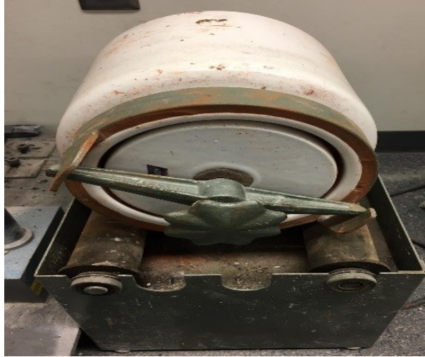
Figure 5-6 Milling the received red mud sample using Rotary Milling Machine
