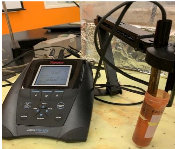
Figure 5-11 Measuring the surface pH value for solid Red Mud sample
