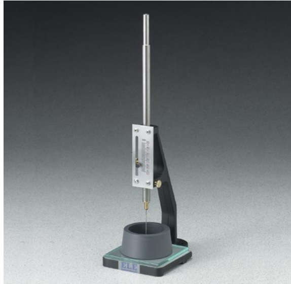
Figure 5-4 Vicat needle apparatus for setting time evaluation
