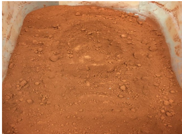
Figure 5-7 Red mud sample after milling inside the Rotary Milling Machine.
