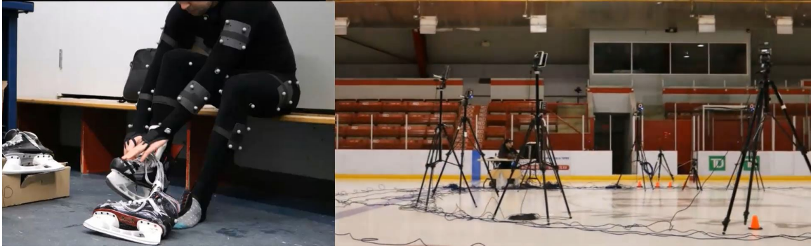
Figure 2.1: An illustration of state-of-art infra-red based motion capture system. Reflective markers are placed on the player and equipment, which were analyzed by the camera system to study the kinematics of the sport [Source: Ice Hockey Research Group, Mcgill University].
