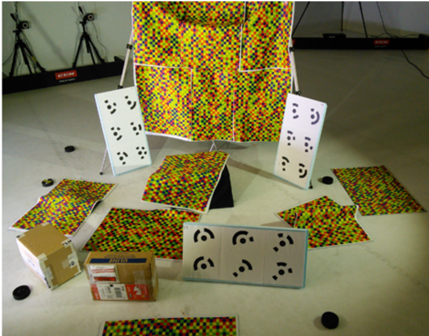
Figure 3.6: An example setup we used for one of the acquisition. For calibration, we use coded circular scale bars and calibration cloth. The color calibration cloth helps to increase the correspondence between the stereo images and give better results.
