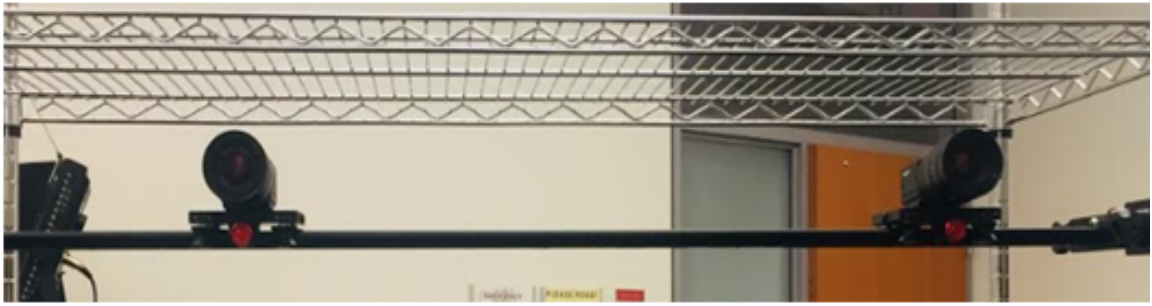
Figure 4.3: An illustration of the fast speed synchronized cameras setup mounted on the portable platform. The distance between the cameras can be changed as required. This system is customized to cater the need of easy portability.
