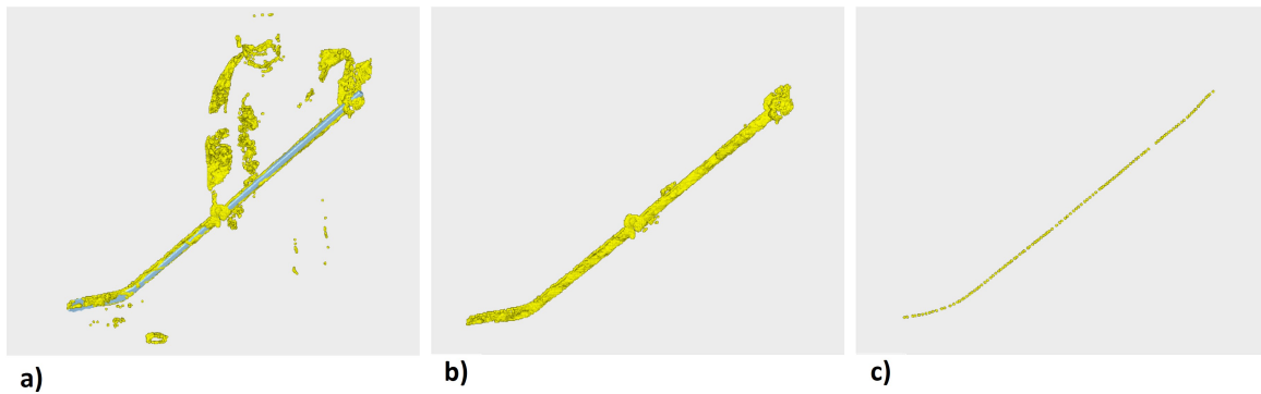
Figure 4.13: Secondary pruning of point cloud with proximity based technique. Figure-a) shows both the pruned point cloud (Yellow) obtained after primary pruning and the initially aligned stick template (Blue). Figure-b) showcases the point cloud after secondary pruning based on proximity with initially aligned stick template. Figure-c) illustrates the Medial axis generated with the final pruned point cloud. By using a secondary proximity based pruning technique all the outliers are removed from the point cloud and a clean Medial axis can be generated.
