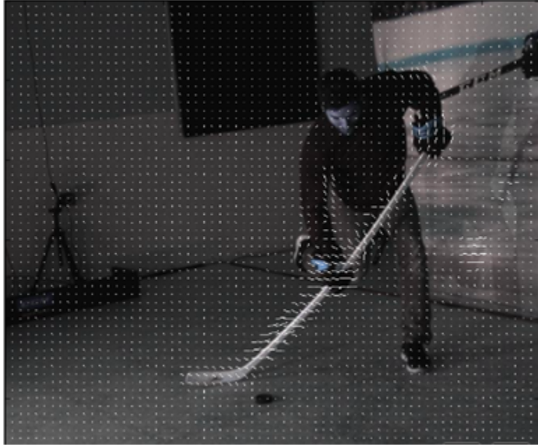
Figure 3.12: Showcasing the vector representation (white lines) of the resultant Dense optical flow calculated using the Farneback's two frame optical flow algorithm with OpenCV. The displacement of pixels observed by the optical flow is vividly visible around the ice hockey stick which is the dominant moving object in the selected image pair.
