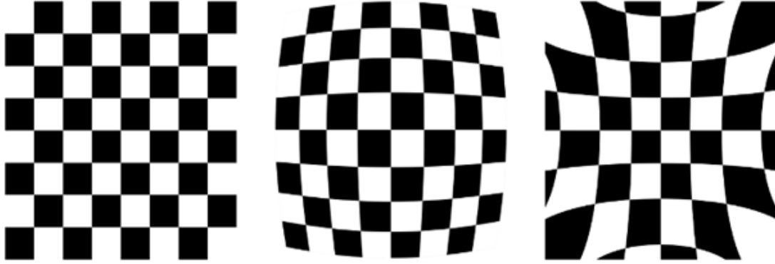
Figure 3.4: Left to right, example showing no-distortion, positive radial and negative radial distortion respectively (courtesy: openCV).
