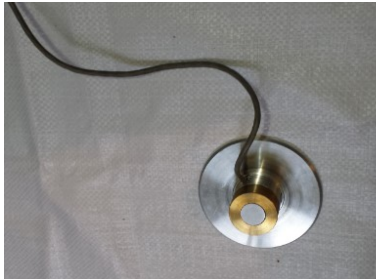
Fig. 3.3. Pressure transducers and its special box
