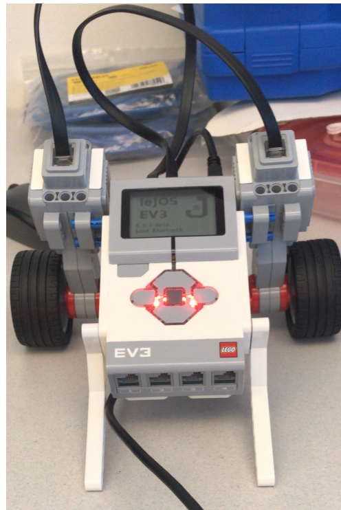
Figure 23. EV3 Robot Built in our Lab for the Proof-of-Concept Prototype from the EV3 LEGO Mindstorms Kit
