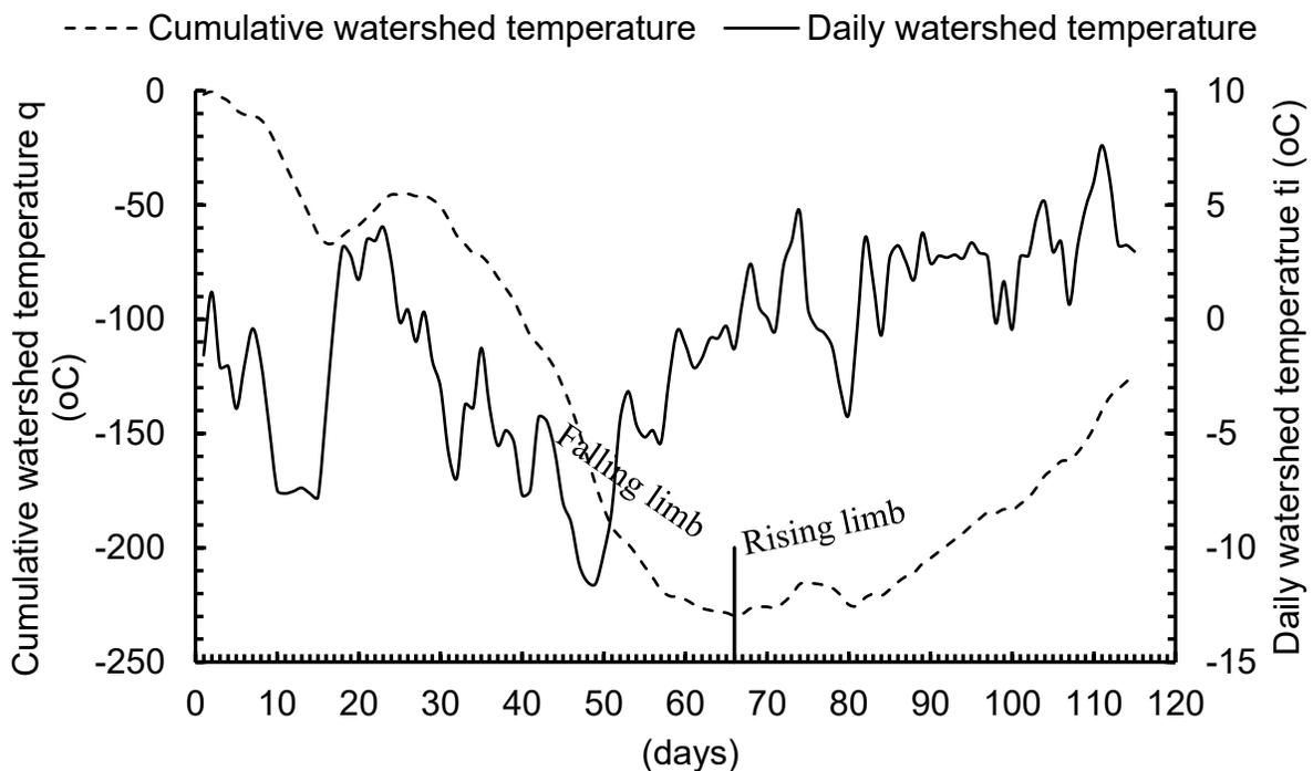
Figure 3.4 Sample division of a hydrological year into falling and rising limbs.
