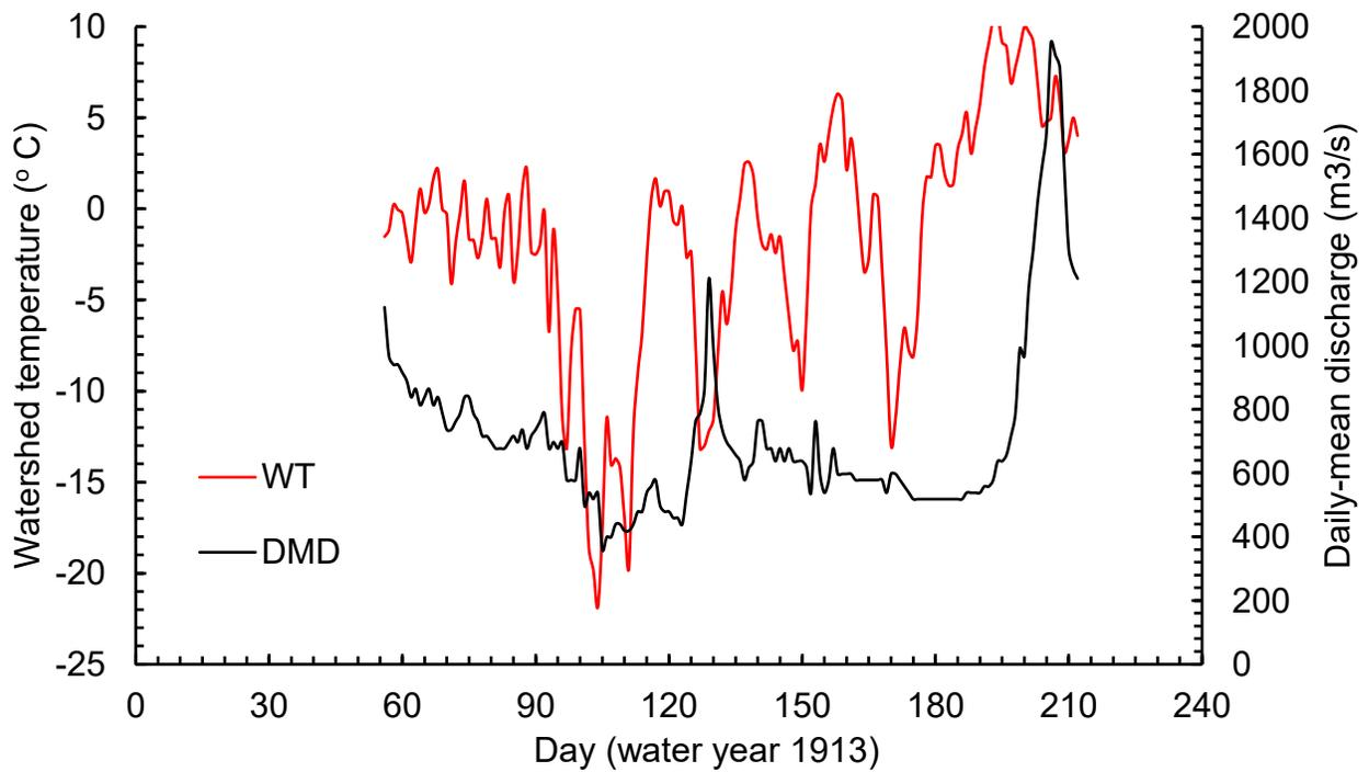
Figure 3.3 Time series of daily mean discharge (DMD) and daily watershed temperature (WT)
