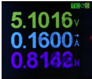
Figure 91: Total power of platform @ send and receive data
