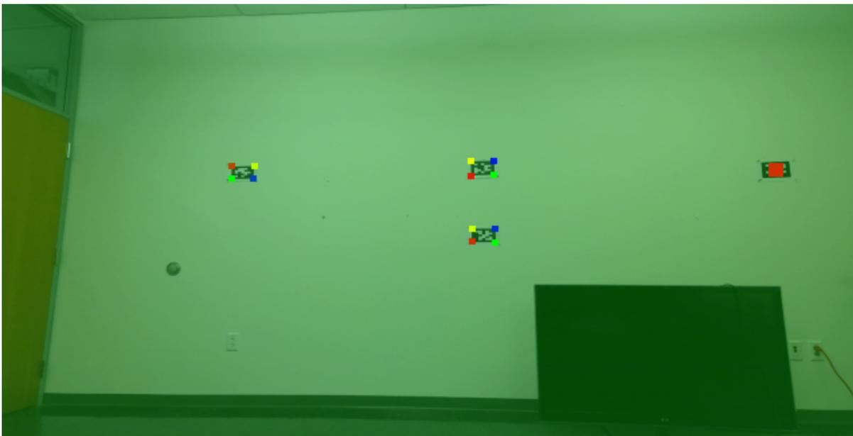
Figure 4.19: Screen turns green if there are markers in the scene and camera pose is within optimum position with respect to the scene (RGB image)
