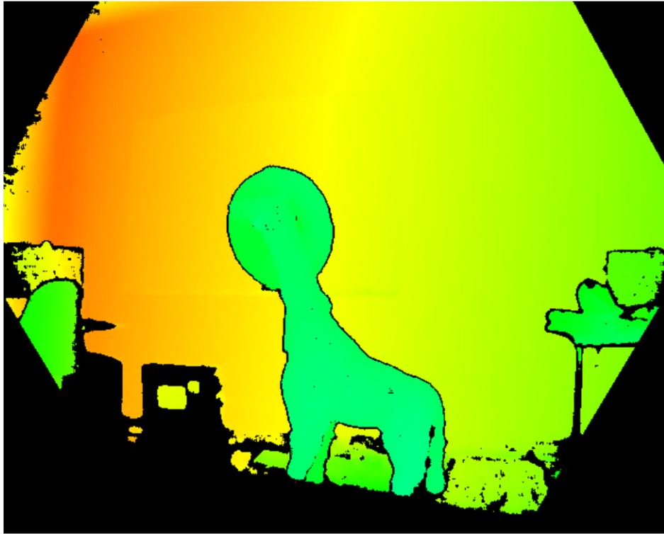
Figure 4.13: Depth image taken from Kinect
