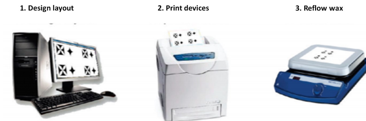
Figure 2-11 Schematics of the fabrication of paper-based analytical devices using the wax printing technique. Adapted from Carrilho et al (Carrilho et al., 2009)
