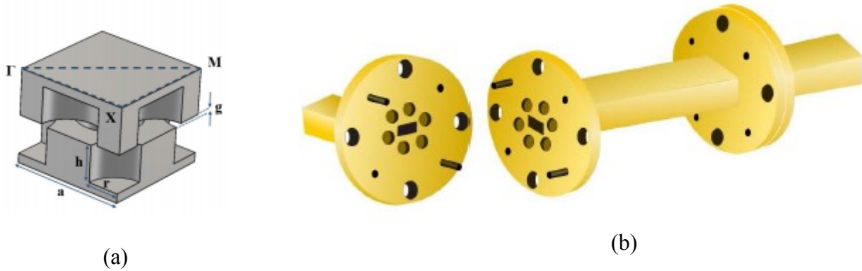
Fig 2.7: Glide-symmetric structure mentioned in [37] (a) Unit cell of a holey glide-symmetric method with dimensions of h = 2 mm and r = 1.4 mm designed for a frequency range of 40-60 GHz and (b) Rectangular waveguide joined to flanges with glide-symmetric holes on both sides
