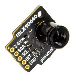
Figure 3.4: MLX90640, 32\*24 pixels thermal camera
