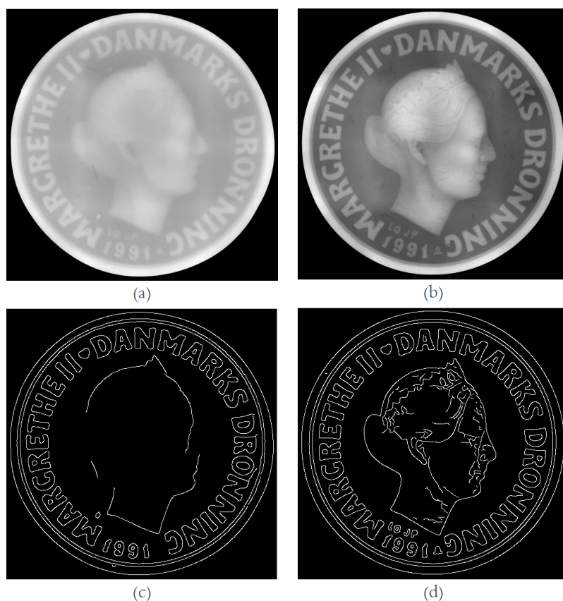
Figure 4-4 Edge detection for two coins with different qualities; (a) a poor quality Danish coin, (b) a good quality Danish coin, (c) and (d) edges detected by Canny for a and b, respectively.
