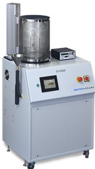
**Figure 3.5** Evaporating Machine at Micro and Nano Device Lab, Concordia University
