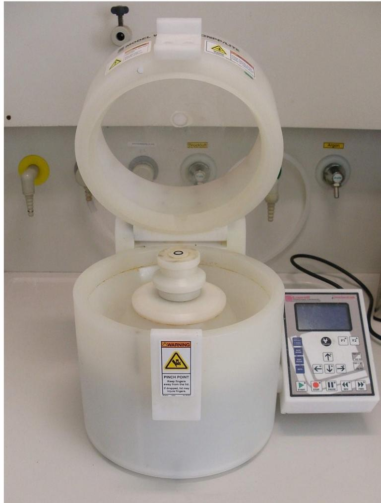
**Figure 3.4** Spin-Coating Device at Micro and Nano Device laboratory, Concordia University
