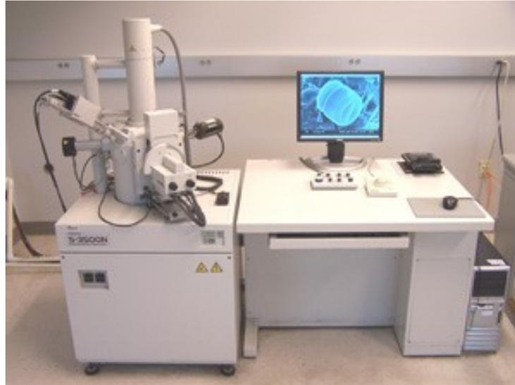
**Figure 3.7** SEM Device at Thermodynamics of Material Research Lab, Concordia University
