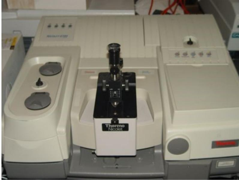
**Figure 3.6** FTIR device at Concordia Center for Composites, Concordia University
